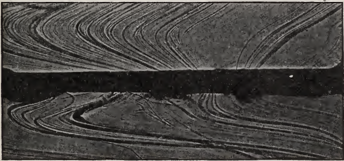
FIG. 1.—Shadowgraph of heavy striæ
