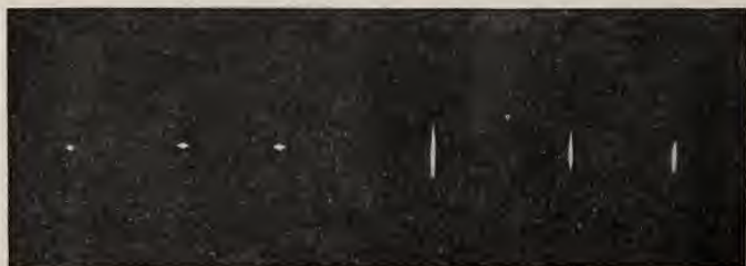
FIG. 15.—(a) Without glass; (b, c) viewed flatwise through rolled window plate (same as Fig. 10); (d, e, f) edgewise through same plate
