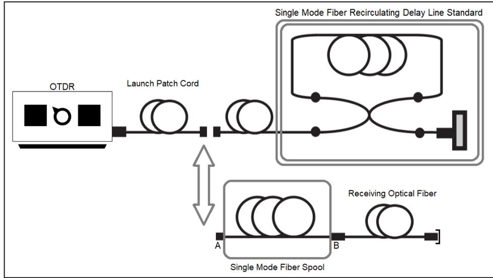
**Fig. 3.** LAMETRO measurement system to realize a pulse propagation delay measurement with an optical time delay reflectometer (OTDR). The delay line standard was previously calibrated at a national metrology institute external to LAMETRO.
