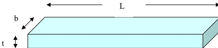
Fig. 2 Diagram of an ideal, rectangular, uniform, fixed-free cantilever
