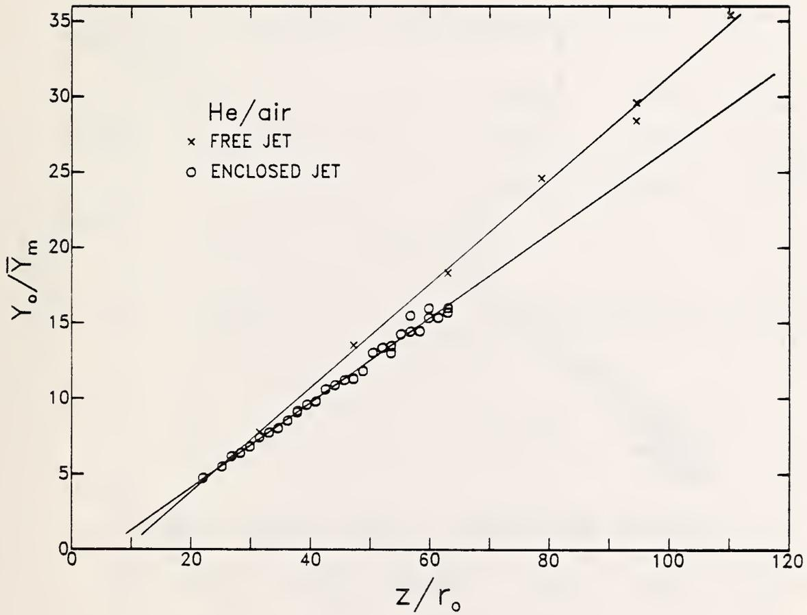
Figure 24. Values of  $Y_o/\bar{Y}_m$  versus  $z/r_o$  are plotted for the helium jet ( $Re = 3950$ ) flowing into both a slow coflow of air and the laboratory. Lines are linear least squares curve fits to the data.
