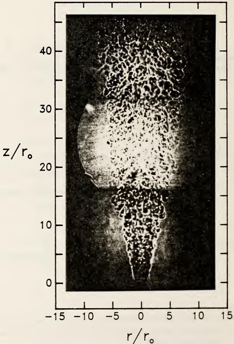
Figure 5. Three shadowgraphs of a turbulent helium jet flowing into a slow coflow of air are superimposed. The Reynolds number for the jet is 3950.
