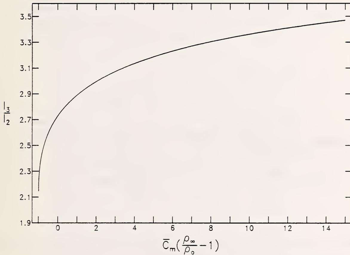
Figure 2. Calculated values for the ratio of the integrals  $I_3$  (eq. 44) and  $I_2$  (eq. (43)) are plotted as a function of  $\bar{C}_m \left( \frac{\rho_\infty}{\rho_0} - 1 \right)$ .
