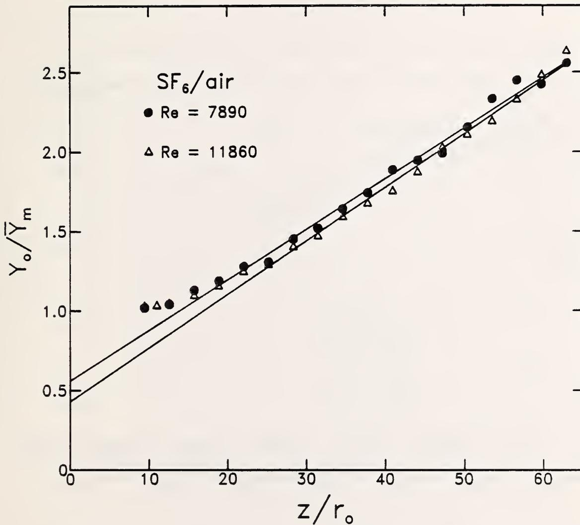
Figure 34. Values of  $Y_0/\bar{Y}_m$  for  $SF_6$  jets at Reynolds numbers of 7890 and 11,860 are shown as functions of  $z/r_0$ . Straight lines represent the results of linear least squares curve fits of the data.
