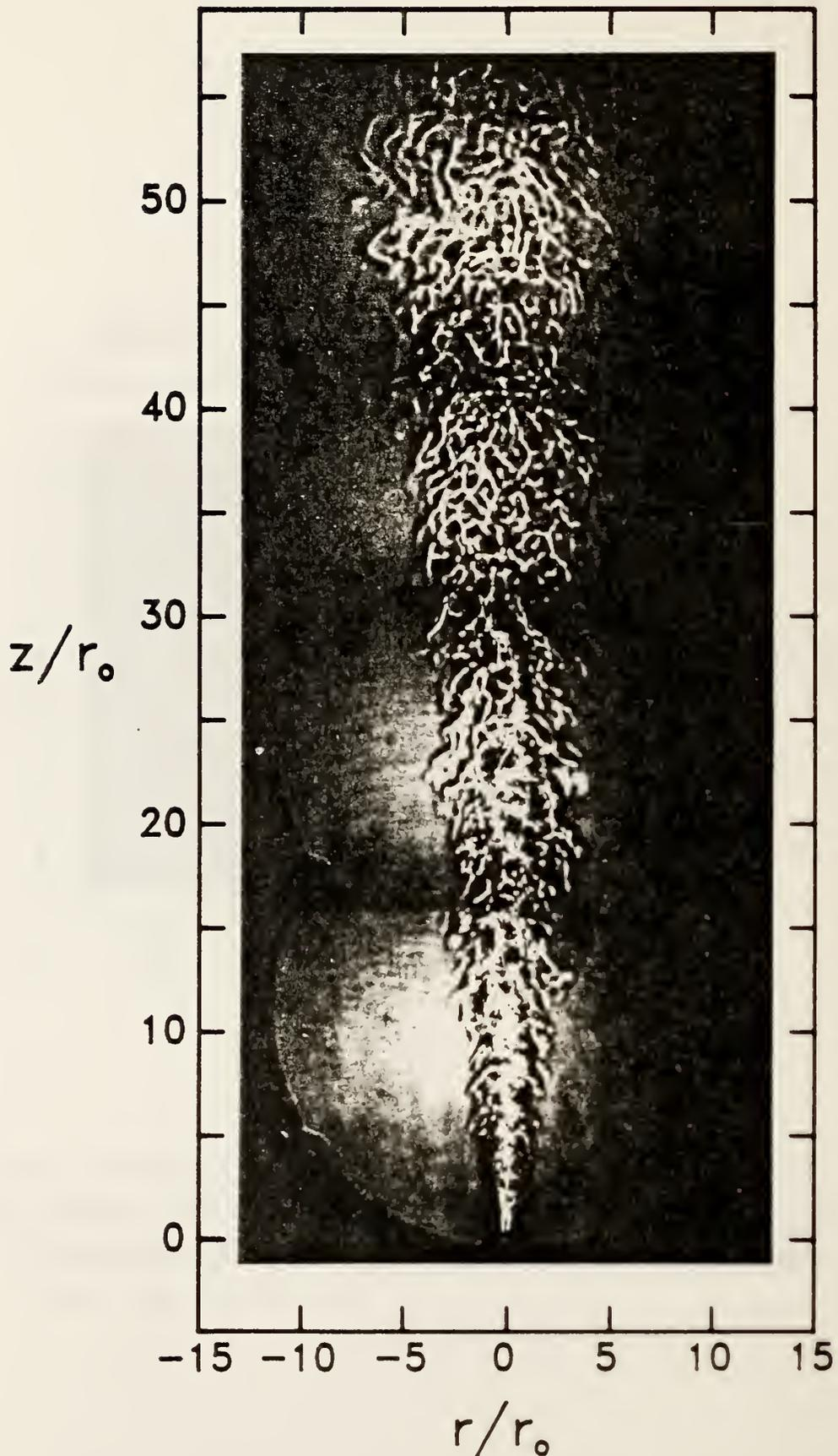
Figure 16. The Reynolds number has been increased to 11,860 for the sulfur hexafluoride turbulent jet entering a slow coflow of air.
