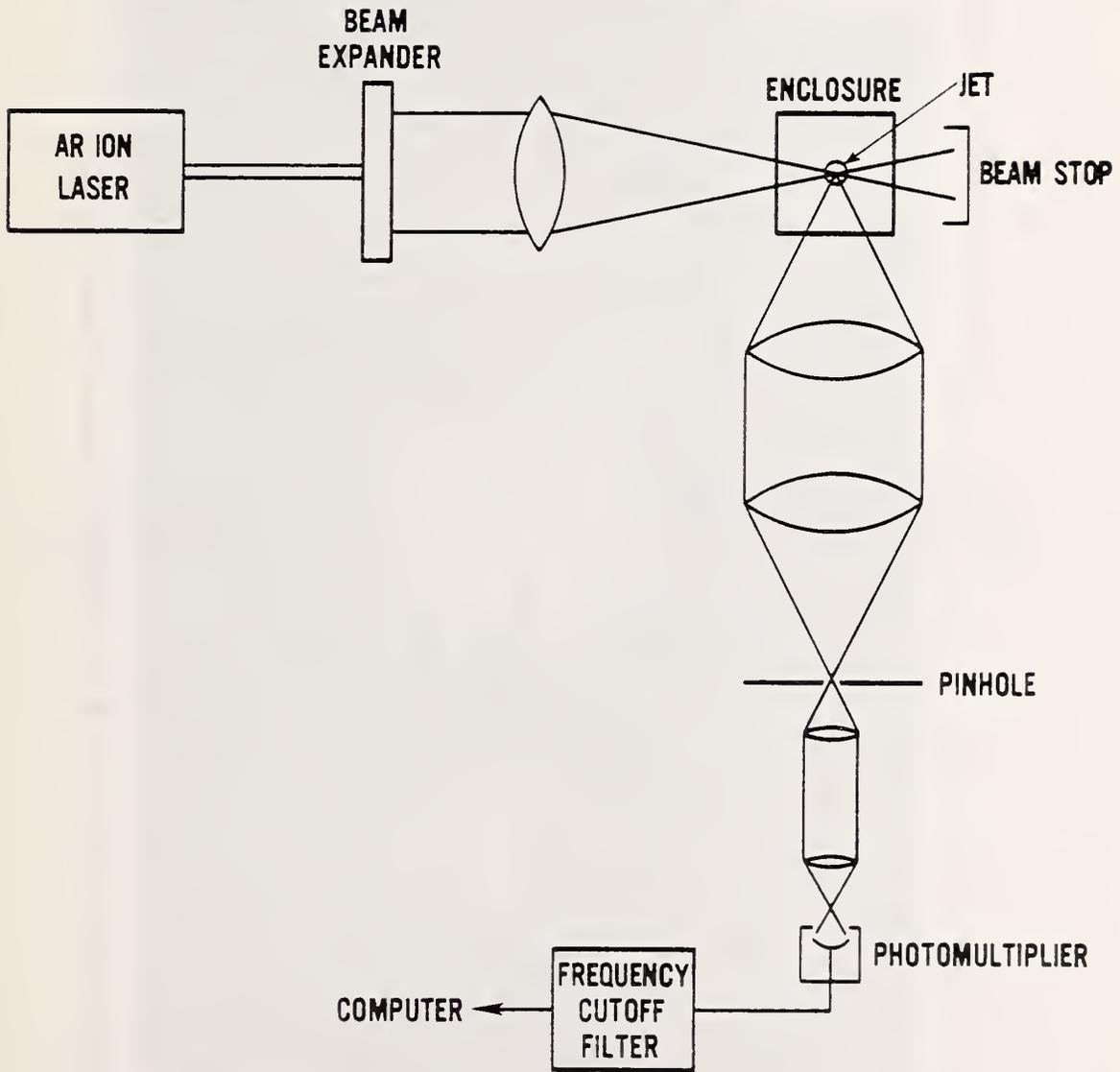
Figure 4. This figure shows the experimental system for making real-time, spatially-resolved, concentration measurements in turbulent flows of binary gas mixtures.
