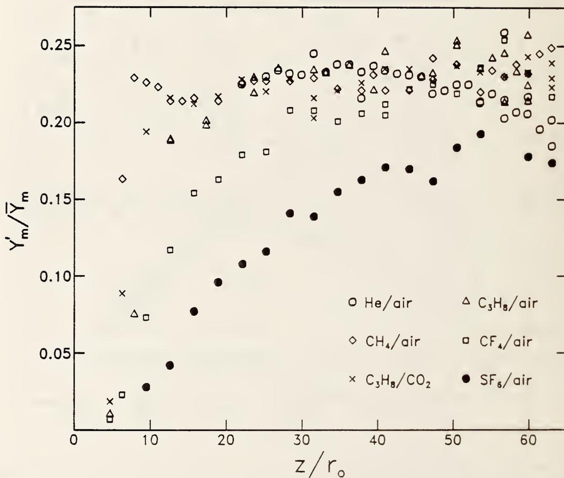
Figure 27. The results of  $Y'_m / \bar{Y}_m$  measurements for the jet/coflow pairs listed are plotted as functions of  $z/r_0$ . Note that the values for each flow approach a common asymptote of  $(Y'_m / \bar{Y}_m)_{\text{asym}} \approx 0.23$ .
