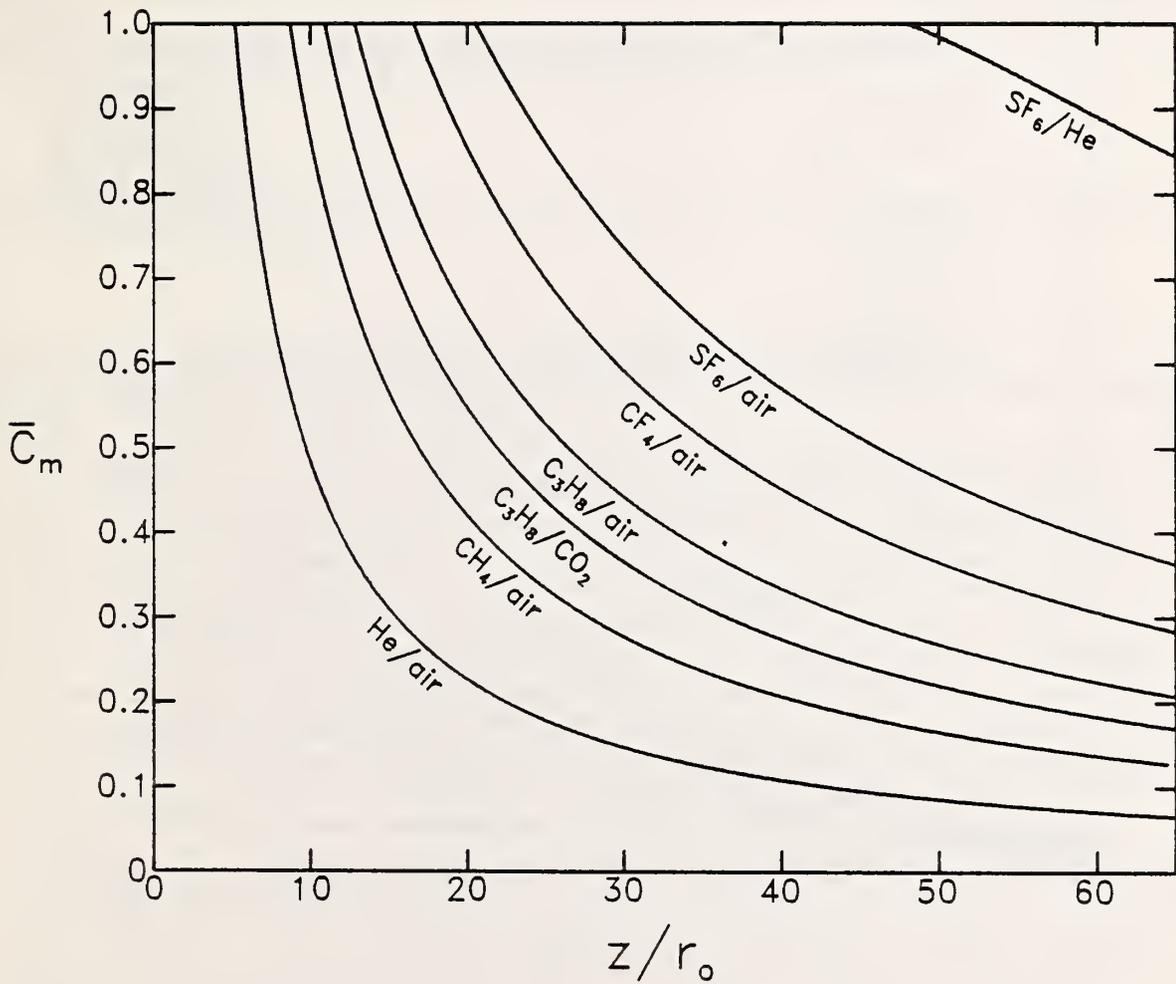
Figure 40. Values of  $\bar{C}_m$  calculated in the manner suggested by Rodi [5,23] are plotted as functions of  $z/r_0$ . Values of jet to surrounding gas density ratios correspond to those used in this study.
