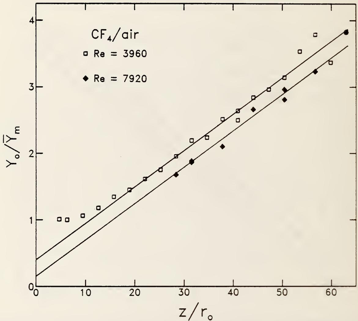
Figure 33.  $Y_o/\bar{Y}_m$  values for two different Re flows of carbon tetrafluoride into air coflows are plotted as functions of  $z/r_o$ . Linear least squares curve fits to the data are represented by the lines.
