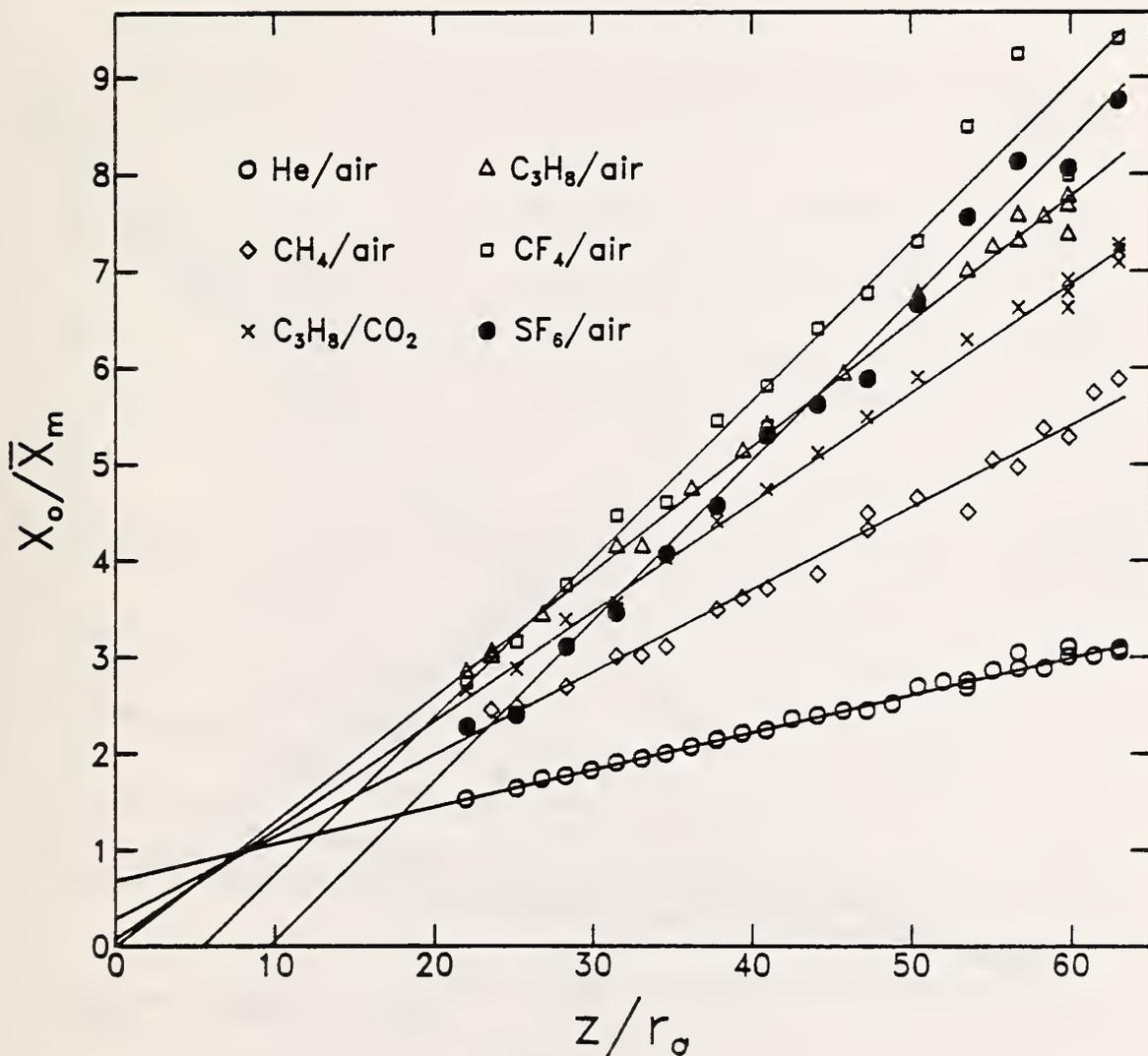
Figure 22. Inverse centerline values of jet gas mole fraction, normalized by multiplying by the jet gas mole fraction ( $X_0 = 1$ ), are plotted as functions of nondimensionalized downstream distance for six different jet/coflow gas pair combinations. Straight lines are linear least squares curve fits of the data.
