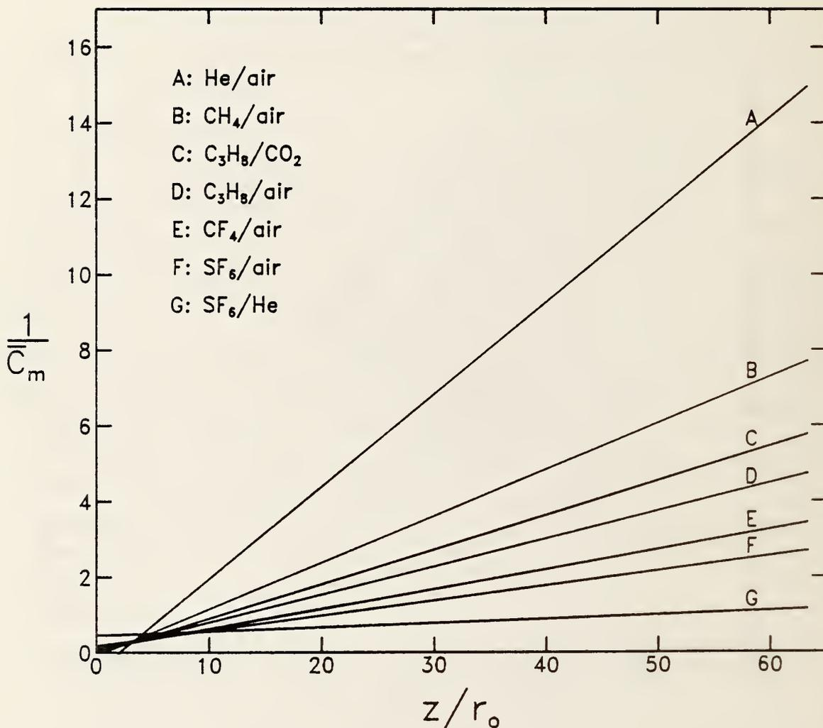
Figure 41. The calculations shown in fig. 40 have been redrawn as  $1/\bar{C}_m$  versus  $z/r_0$ . Comparison of this figure with fig. 39 shows that the approximate treatments of Thring and Newby [18] and Rodi [5,23] give similar predictions for the dependence of average centerline concentration falloff on the jet/coflow gas density ratio.
