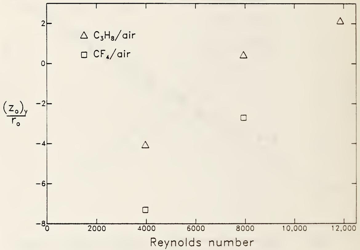
Figure 35. Virtual origins which are obtained from centerline concentration measurements in the C<sub>3</sub>H<sub>8</sub>/air and CF<sub>4</sub>/air flows are plotted as functions of jet Reynolds number.
