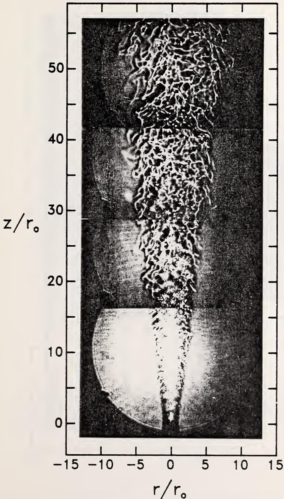
Figure 11. Four superimposed shadowgraphs are shown for a turbulent jet of propane ( $Re = 11,880$ ) entering a slow coflow of air.
