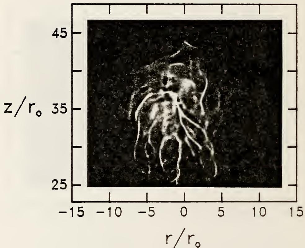
Figure 19. The fountain formed by the SF<sub>6</sub> jet (Re = 3950) entering into helium can be clearly seen in this shadowgraph recorded for downstream distances extending from  $z/r_0 = 25$  to 47.
