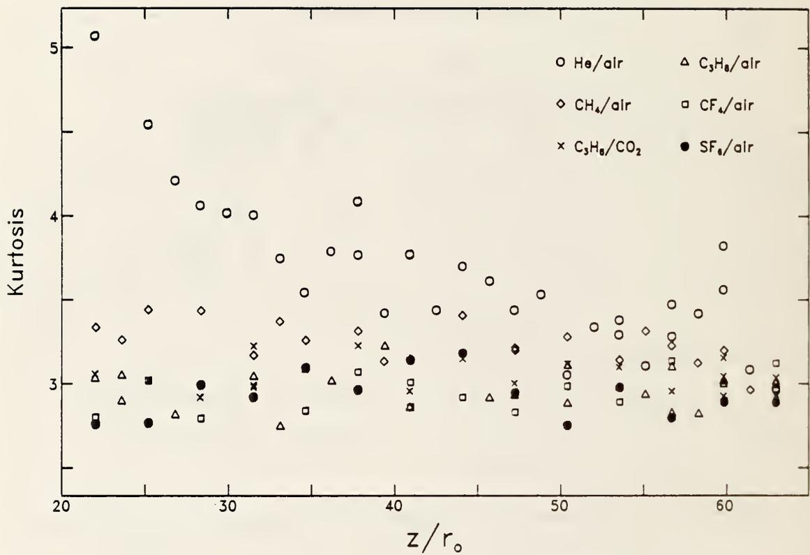
Figure 31. Kurtosis values for centerline concentration fluctuations are plotted as functions of  $z/r_0$  for the jet/coflow gas pairs listed.
