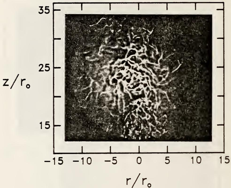
Figure 13. A shadowgraph for the same flow described in fig. 12 is shown at larger downstream distances. Again, jet gas is observed in locations well outside of the jet.
