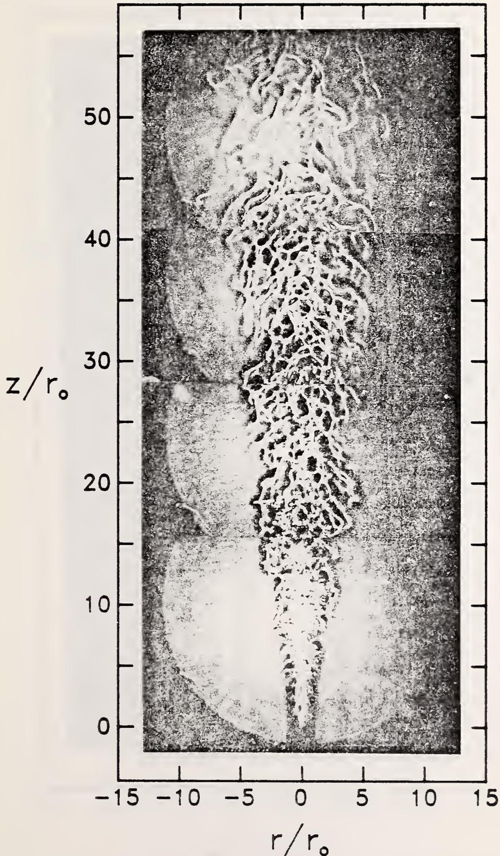
Figure 9. Shadowgraphs of the same propane jet visualized in fig. 8, but flowing into a slow coflow of air, are shown.
