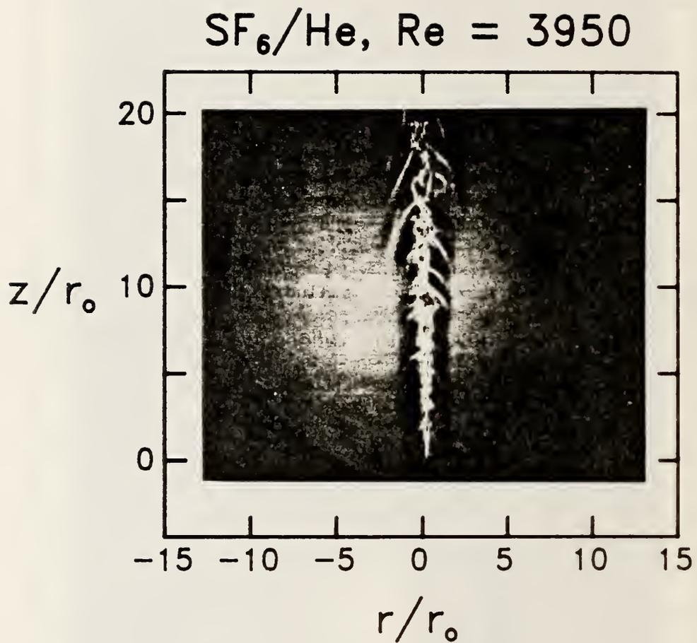
Figure 17. The near field region of a  $\text{SF}_6$  jet ( $\text{Re} = 3950$ ) flowing into a slow coflow of helium is visualized by shadowgraphy.
