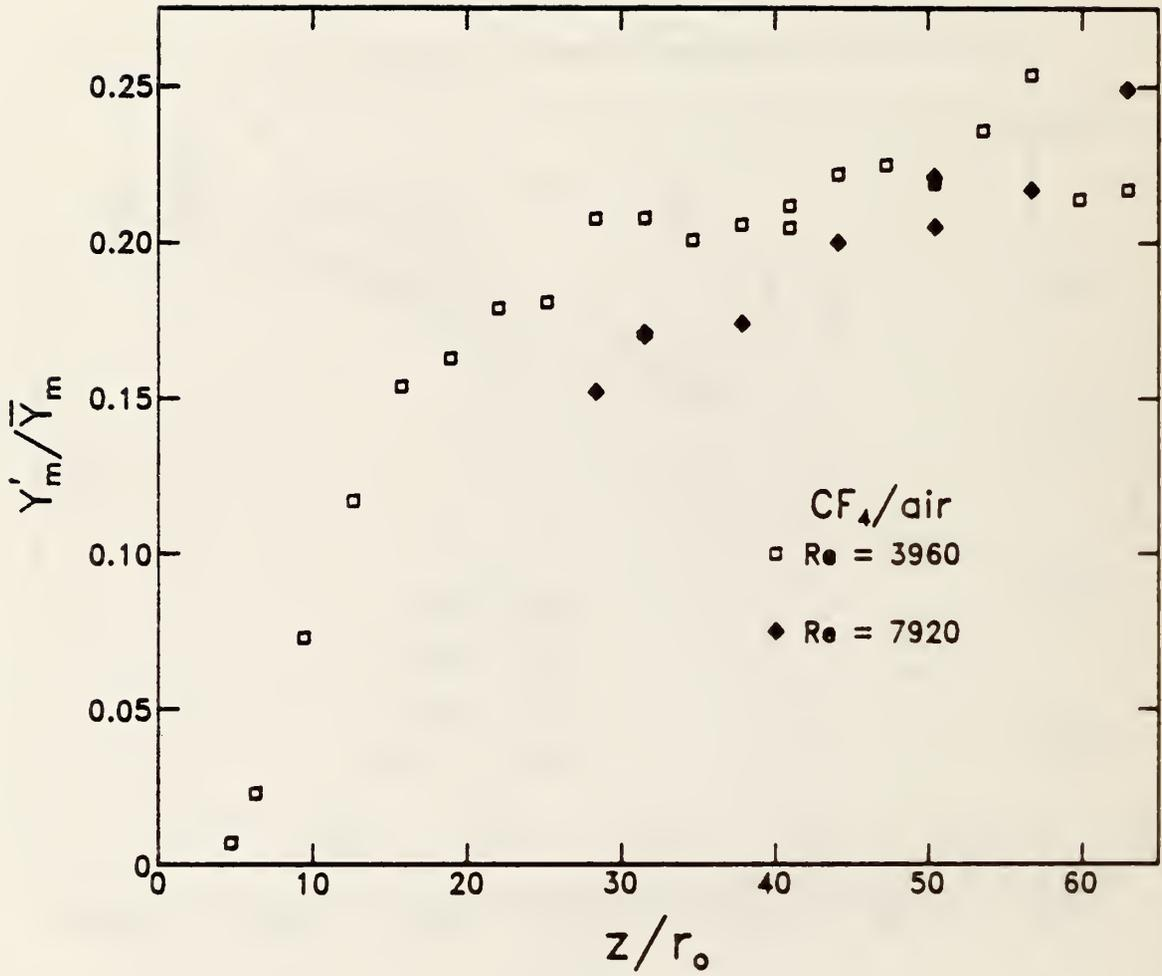
Figure 37. Mass fraction unmixedness values are plotted as functions of  $z/r_0$  for two different  $Re$  jets of  $CF_4$  flowing into slow air coflows.
