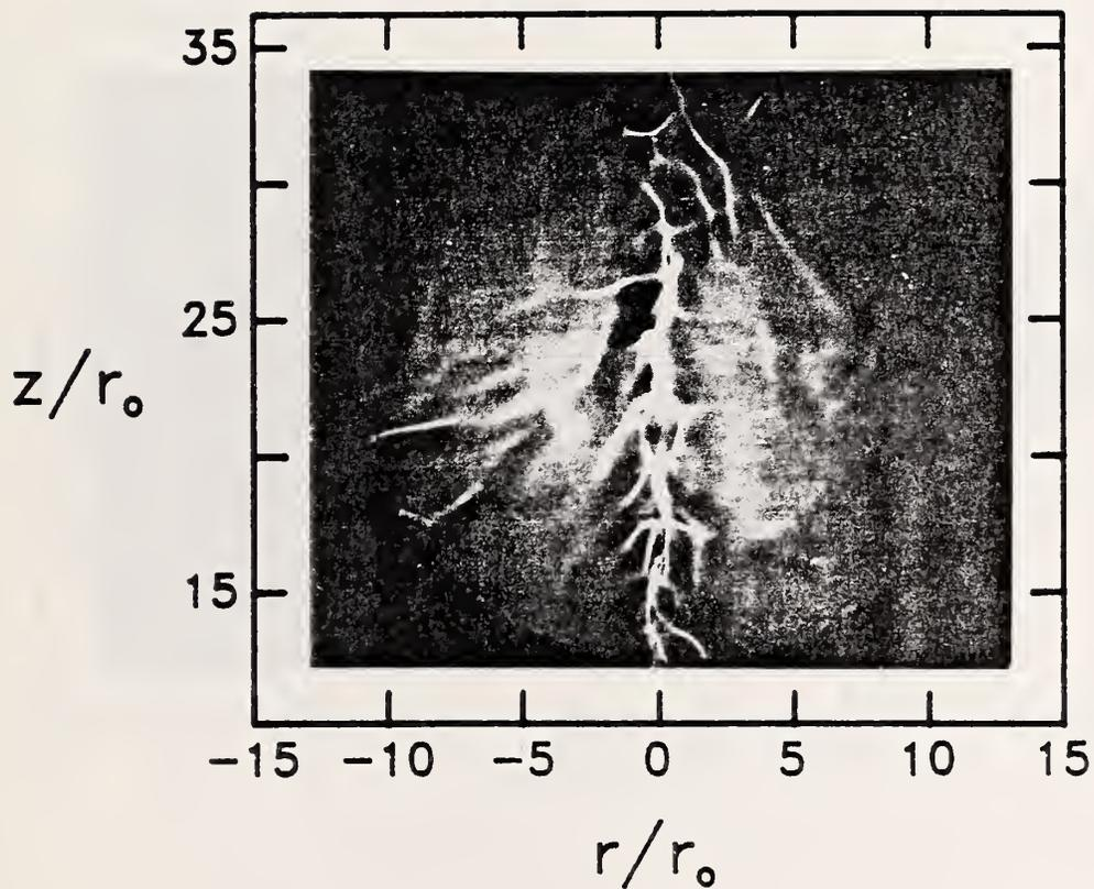
Figure 18. A shadowgraph centered at  $z/r_0 \approx 24$  is shown for the  $\text{SF}_6$  jet of  $\text{Re} = 3950$  flowing into a slow coflow of helium.
