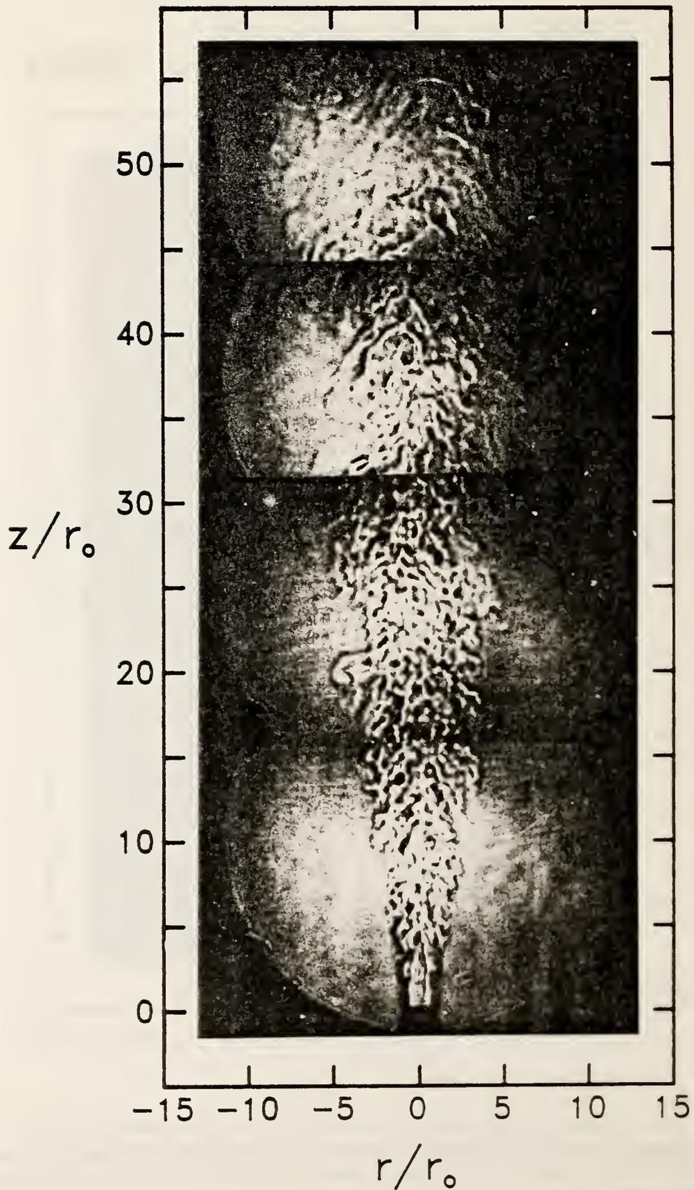
Figure 8. The superposition of four shadowgraphs is shown for a turbulent jet of propane flowing into a slow coflow of carbon dioxide. The Reynolds number for the jet is 3960.
