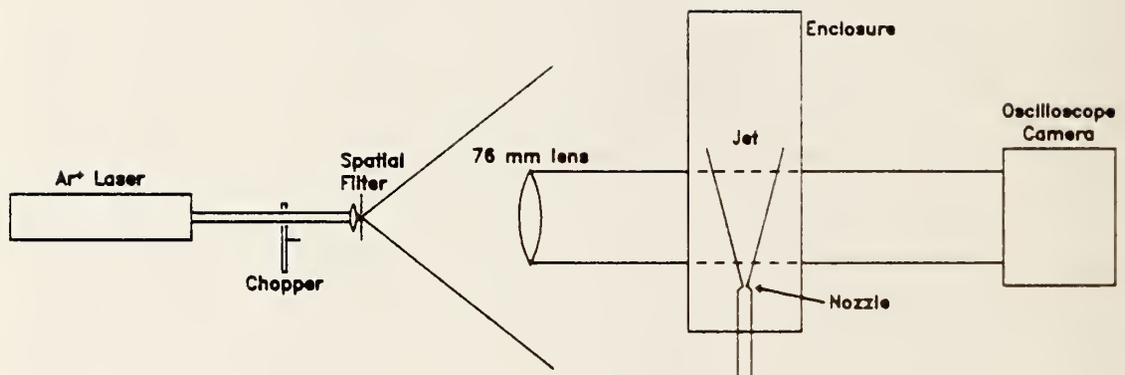
Figure 3. The experimental arrangement employed for time-resolved shadowgraphy of variable density flows is shown.
