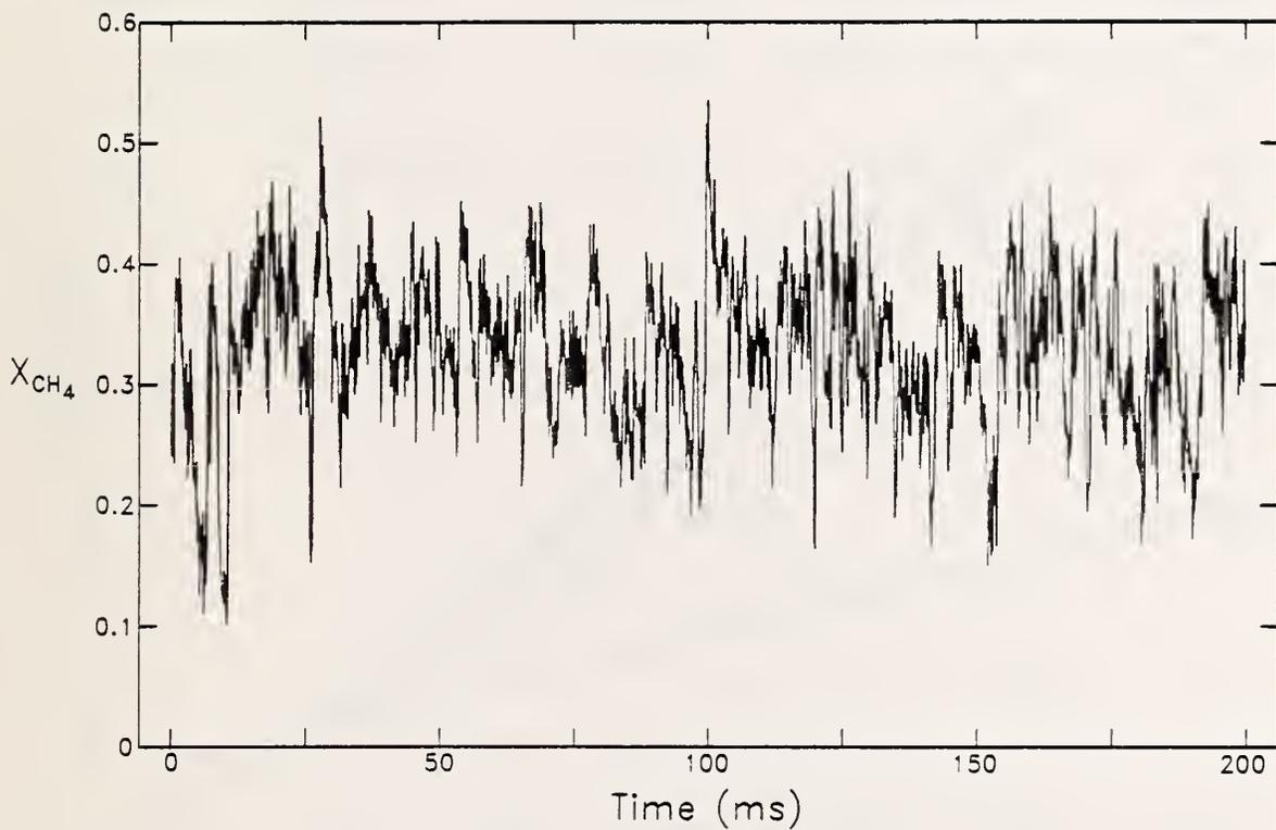
Figure 20. A portion of the time-resolved methane concentration fluctuations within a turbulent jet of methane ( $Re = 3950$ ) flowing into a slow coflow of air is shown. The measurements were made on the centerline at  $z/r_0 = 31.5$ .
