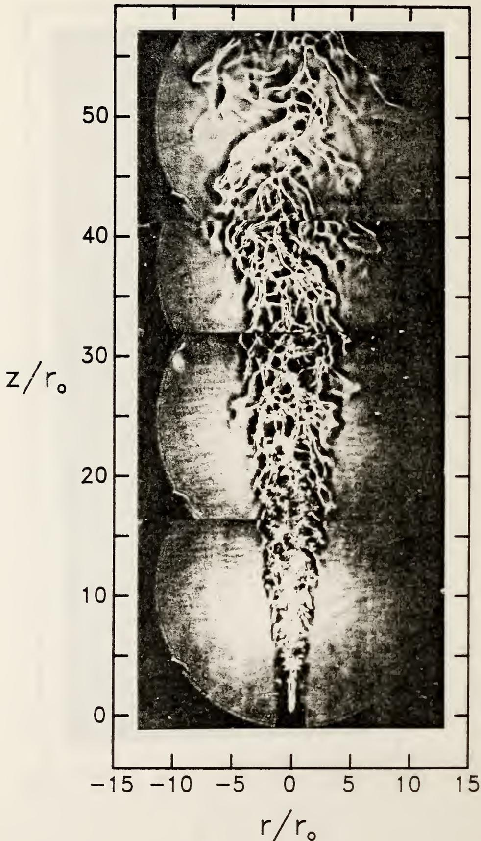
Figure 10. The Reynolds number of the propane jet shown in fig. 9 has been increased to 7930 for the four shadowgraphs which have been superimposed. The coflow gas is again air.
