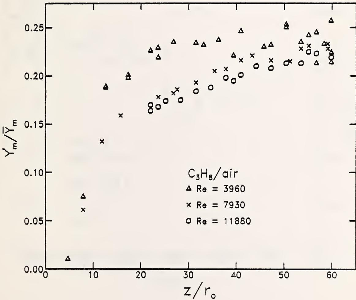
Figure 36. Mass fraction unmixedness values are plotted as functions of  $z/r_0$  for three different Re jets of propane entering slow coflows of air.
