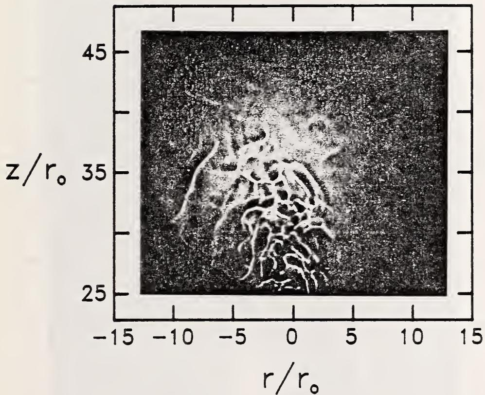
Figure 14. The formation of a fountain by the strongly negatively buoyant jet of  $\text{SF}_6$  ( $\text{Re} = 3950$ ) flowing into a coflow of air is visualized by shadowgraphy. The range of downstream distances extends from  $z/r_0 = 25$  to 47.
