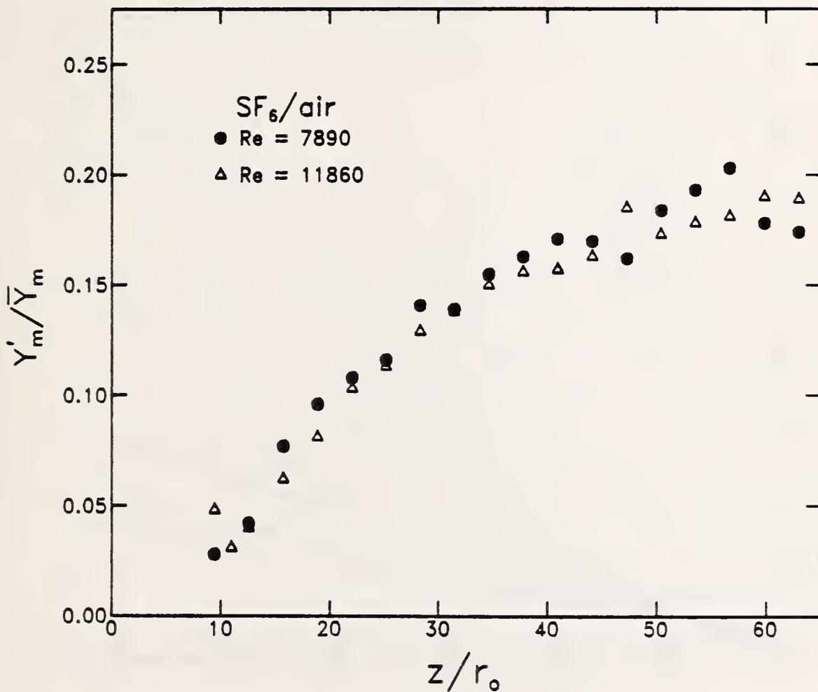
Figure 38. Unmixedness values for jets of  $SF_6$  at Reynolds numbers of 7890 and 11,860 are plotted as functions of  $z/r_0$ . The coflow gas is air.
