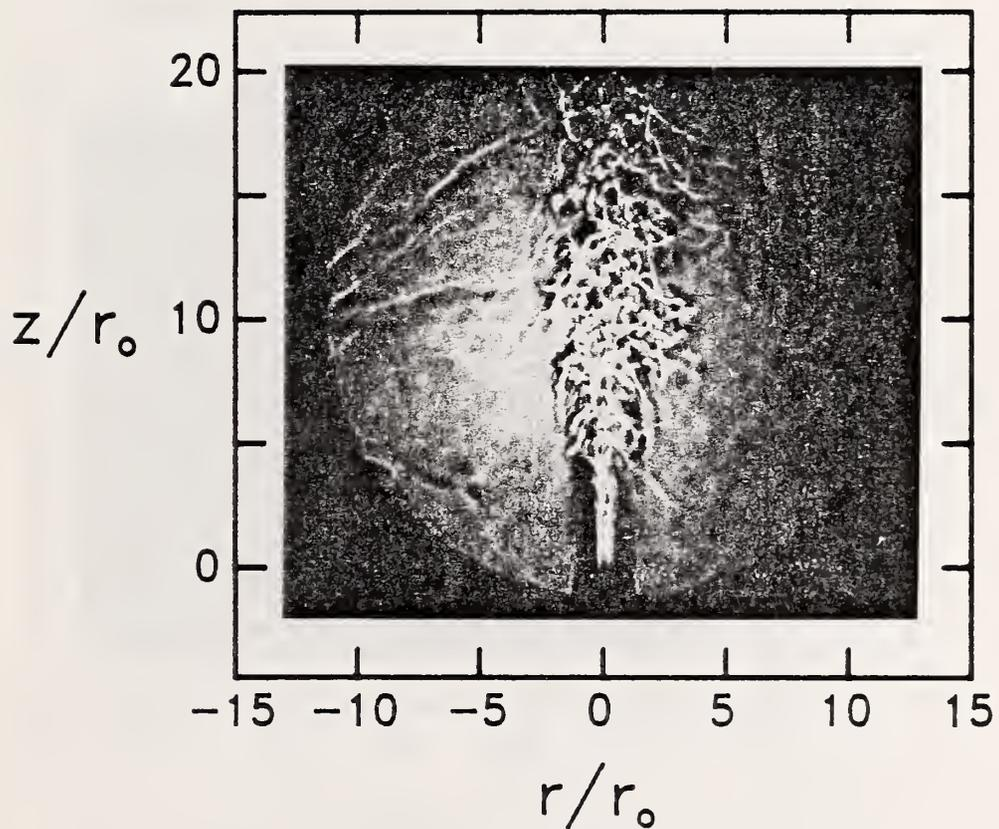
Figure 12. The near-field region of a sulfur hexafluoride turbulent jet (Re = 3950) is visualized by shadowgraphy. Note the presence of jet fluid in regions well outside of the jet.
