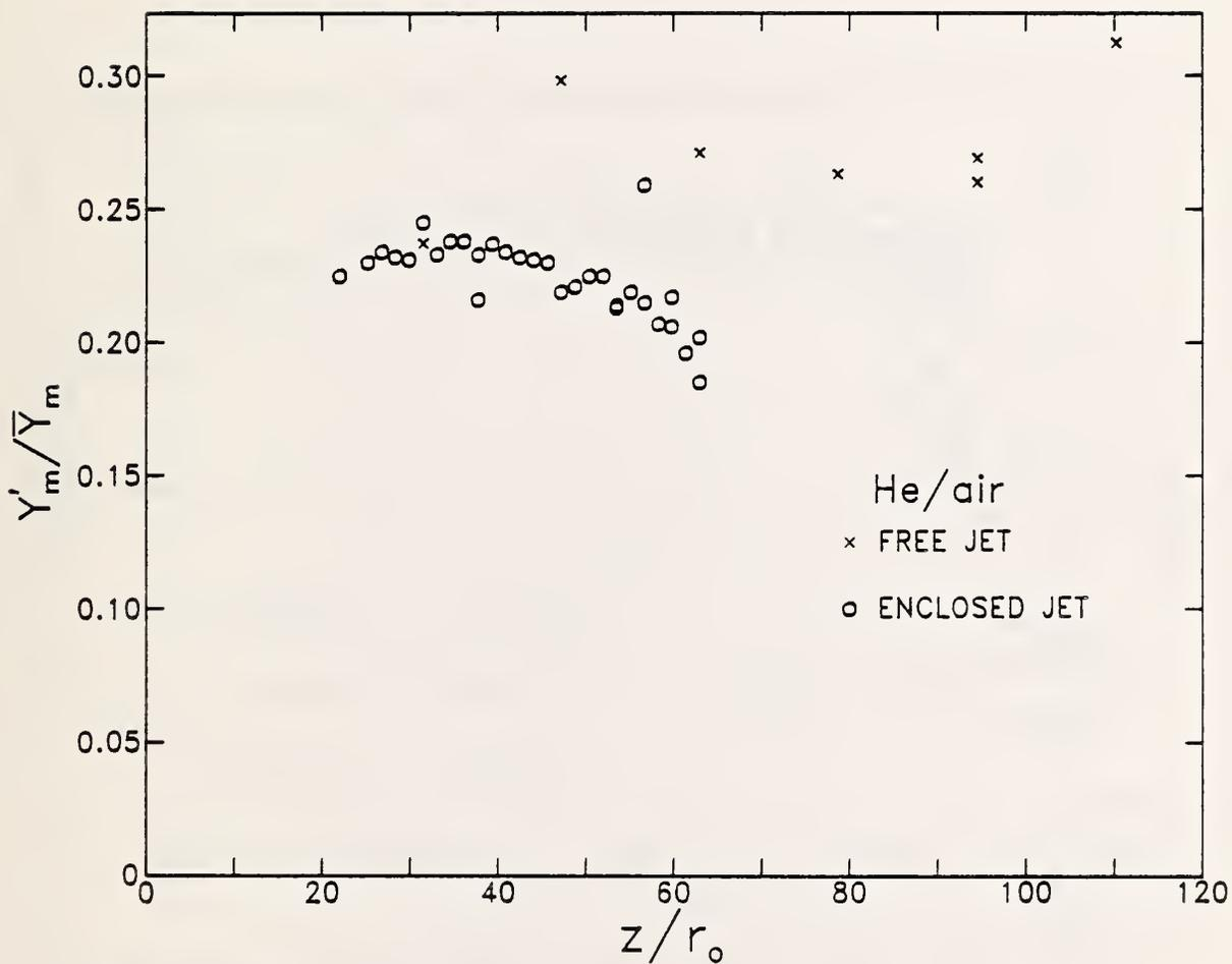
Figure 28. Values of  $Y'_m / \bar{Y}_m$  are plotted as functions of  $z/r_0$  for the helium jet ( $Re = 3950$ ) flowing into a coflow of air and into the laboratory (free jet).
