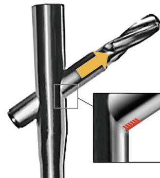
**Fig. 2:** Diagrammatic representation showing repetitive, linearly arranged, regularly spaced transverse scratch marks (red lines) made on the inferior ridge at the intramedullary nail–FNE interface as the FNE migrates medially.
