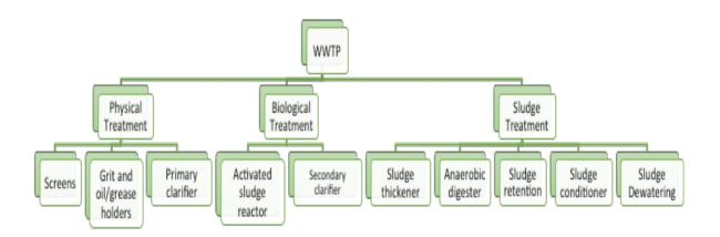
Figure 1. Units of urban wastewater treatment plant.
