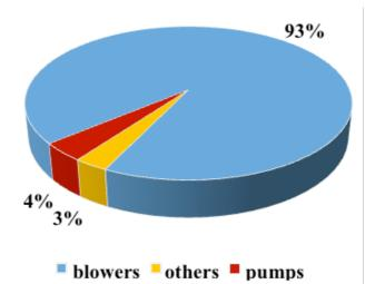
Figure 1. Electricity consumption percentages of some equipment in the activated sludge unit
