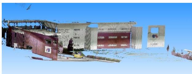
Figure 2. OS Explorer House mesh and point cloud from a Leica MS60 Multistation
