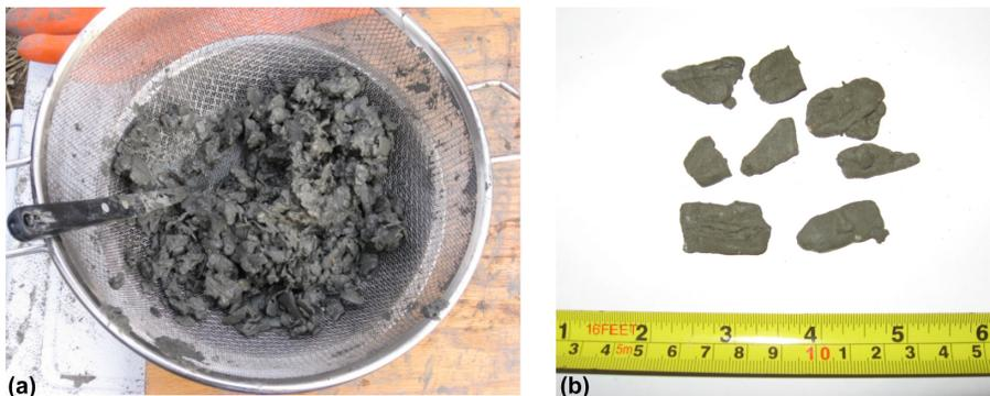
**Figure 3.** Evaluation of core cuttings as an alternative sample source for DVE-LS: **(a)** sieved chip samples after washing, and **(b)** wiped chip samples (typically 25 mm × 15 mm) prior to placement in Ziploc™ bags.
