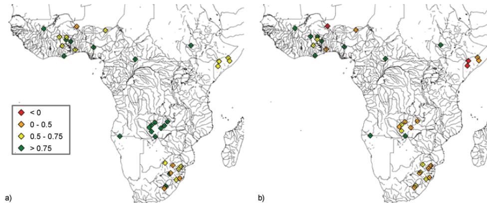
**Figure 5.** Modified Kling-Gupta efficiencies between daily LISFLOOD simulated and observed discharge for **(a)** the calibration period 2004–2008 and **(b)** the validation period 1998–2003.
