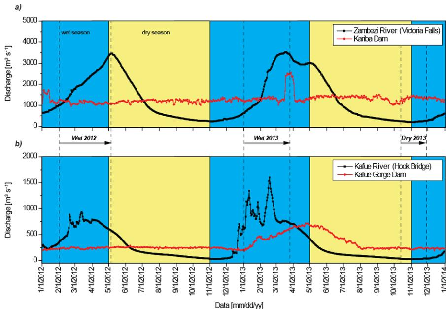
**Figure 2.** Water discharge for: **(a)** the Zambezi River at Victoria Falls power station and the disturbance of natural flow pattern by dam operation at Kariba Dam, and **(b)** for the Kafue River at the Hook Bridge (upstream of the Itezhi Tezhi Reservoir) and the regulated flow at the Kafue Gorge Dam between January 2012 and January 2014 (data from Zambia Electricity Supply Corporation Limited, ZESCO).
