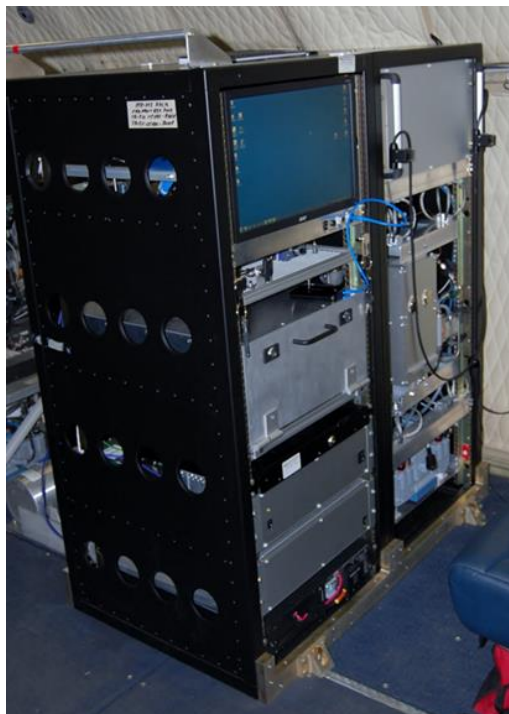
Figure S1. Photograph of the airborne PTR-ToF-MS instrument
