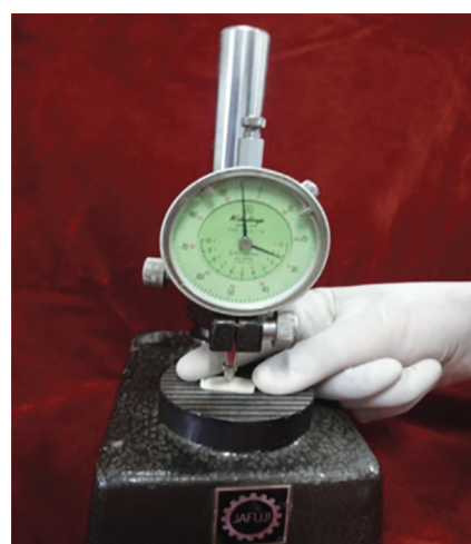
Fig. 6: Surface roughness measured with the help of micron dial indicator
