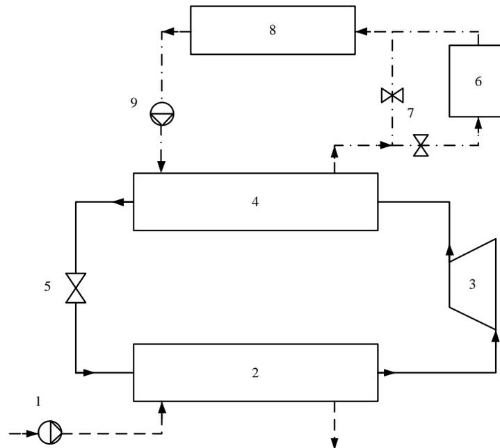
**Figure 1.** A diagram of a heat supply system based on the HP: 1 – pump; 2 – evaporator; 3 – compressor with electric drive; 4 – condenser; 5 – thermostatic valve; 6 – electric boiler; 7 – regulating water valves; 8 – heating devices; 9 – circulation pump of a heat supply system
