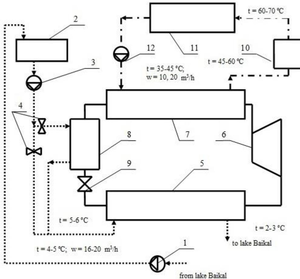
**Figure 3.** The schematic diagram of the Baikal Museum's heat supply system:
