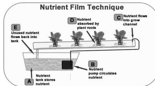
Figure 1: NFT system as plants grow and nutrient circulated in a thin film through plants roots (Shrethsa, 2010).
