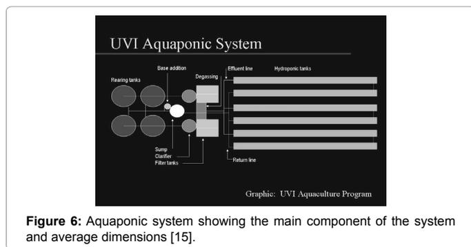
Figure 6: Aquaponic system showing the main component of the system and average dimensions [15].
