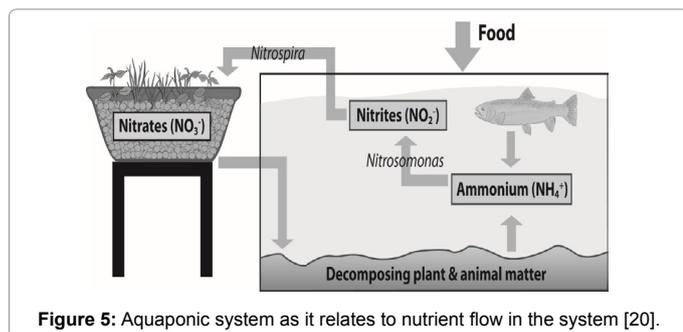
Figure 5: Aquaponic system as it relates to nutrient flow in the system [20].
