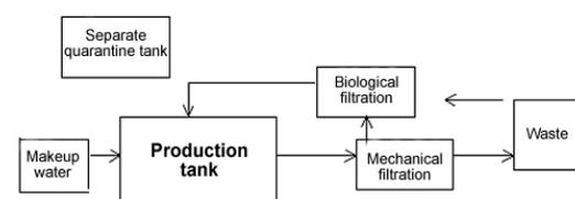
Figure 4: Recirculating aquaculture system as it relates to system setup and design.
