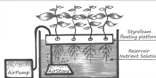
Figure 2: Floating raft system as plants grows on nutrient solution (Shrethsa, 2010).
