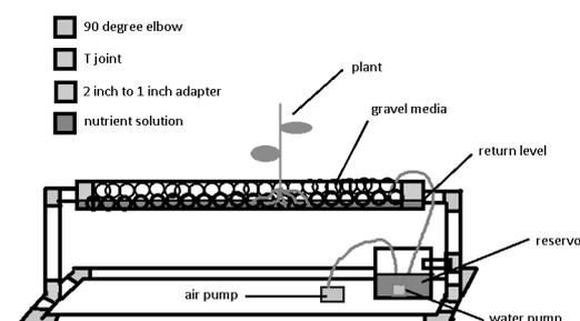
Figure 3: Growth medium bed system as plant raised in growth beds and nutrients circulated flow through the FAO [2].
