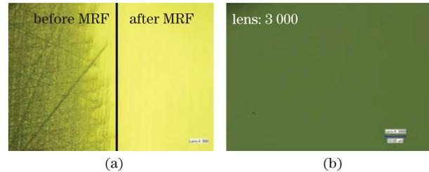
Fig. 3. KDP surface appearances after polishing. (a) Comparison of surface before and after MRF and (b) KDP surface micro-shape after MRF.
