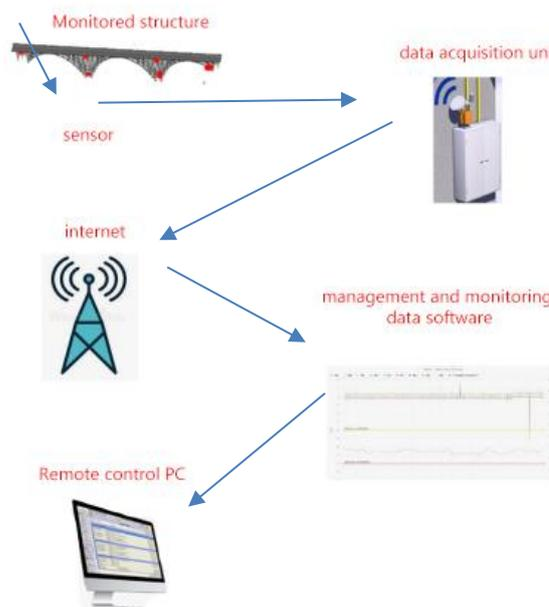
Fig.15 - Data transmission, from sensors to software.
