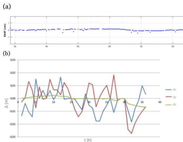
Fig.9– GPS monitoring results: (a) pillar, (b) central span.
