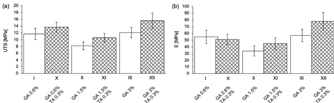
Fig. 4. Increase in (a) UTS values by 17% to 29% and (b)  $E$  values by 32% (series XI) and 37% (XII) noted after TA additional cross-linking
