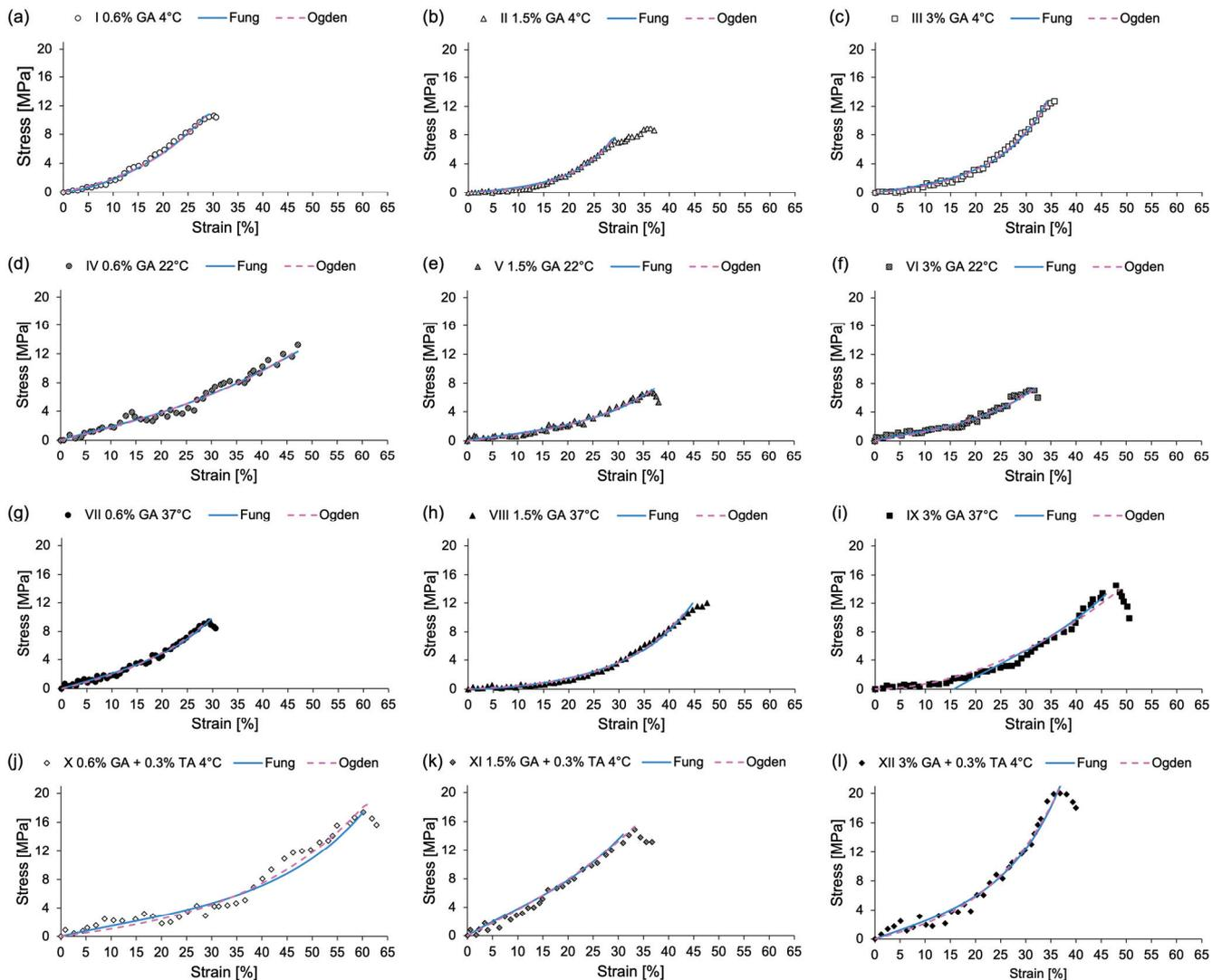
Fig. 5. Stress–strain curves obtained for cross-linked samples of pericardium and fitted by Fung's model and Ogden's model
