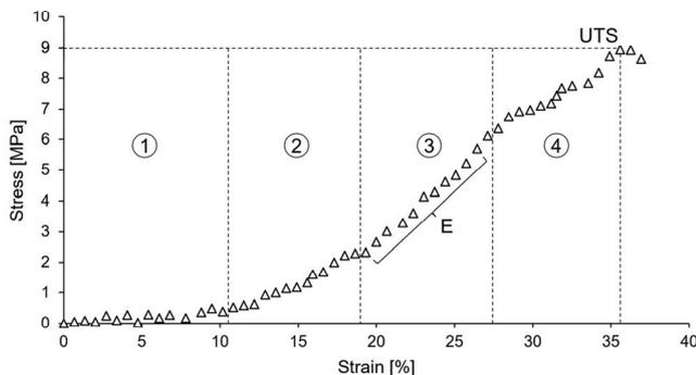
Fig. 2. Stress–strain curve for sample cross-linked with 1.5% GA at 4 °C.
