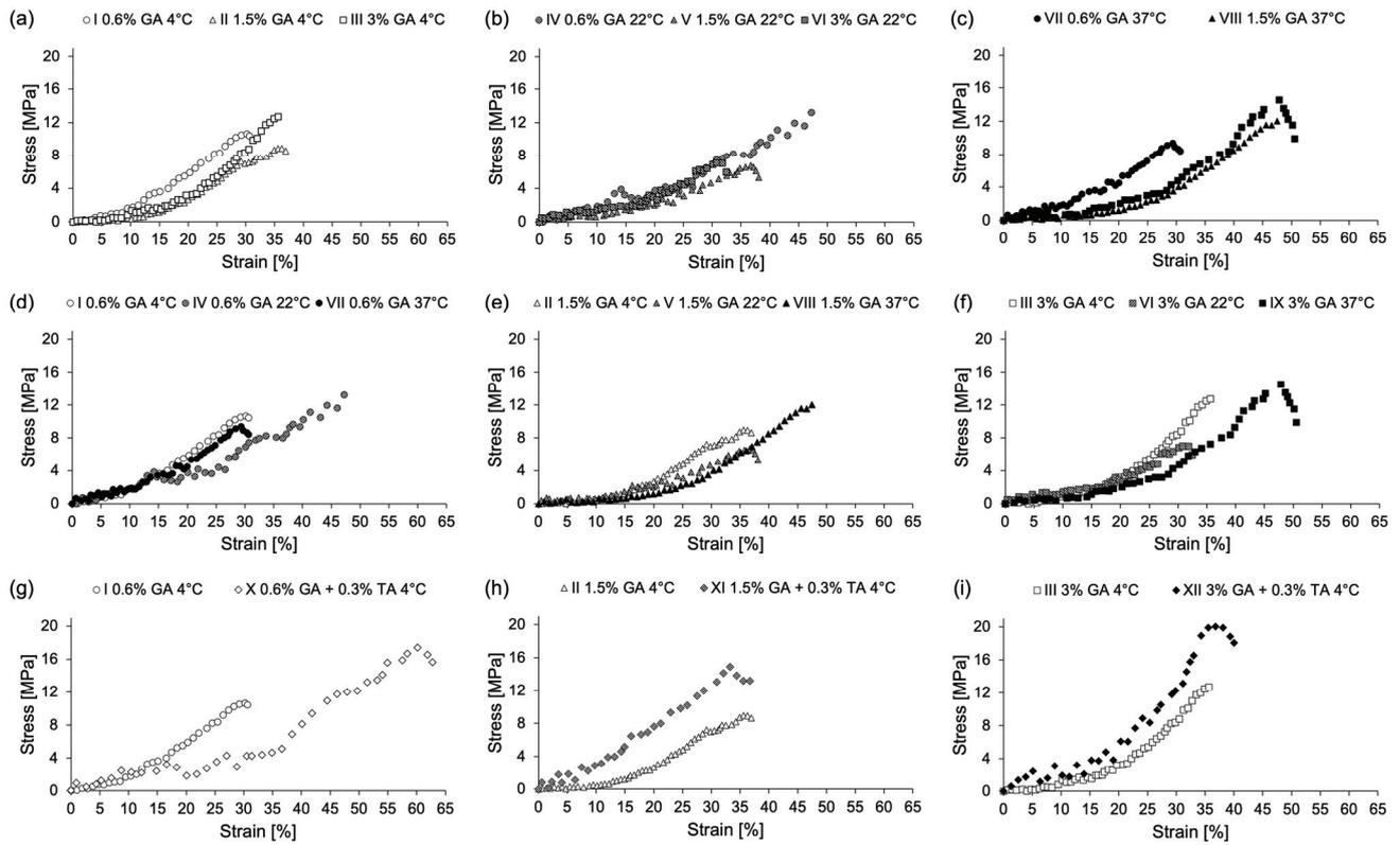
Fig. 3. The stress–strain curves for specimens cross-linked in: (a) 4 °C; (b) 22 °C; (c) 37 °C; (d) 0.6% GA; (e) 1.5% GA; (f) 3% GA; (g) 0.6% GA + 0.3% TA; (h) 1.5% GA + 0.3% TA; (i) 3% GA + 0.3% TA
