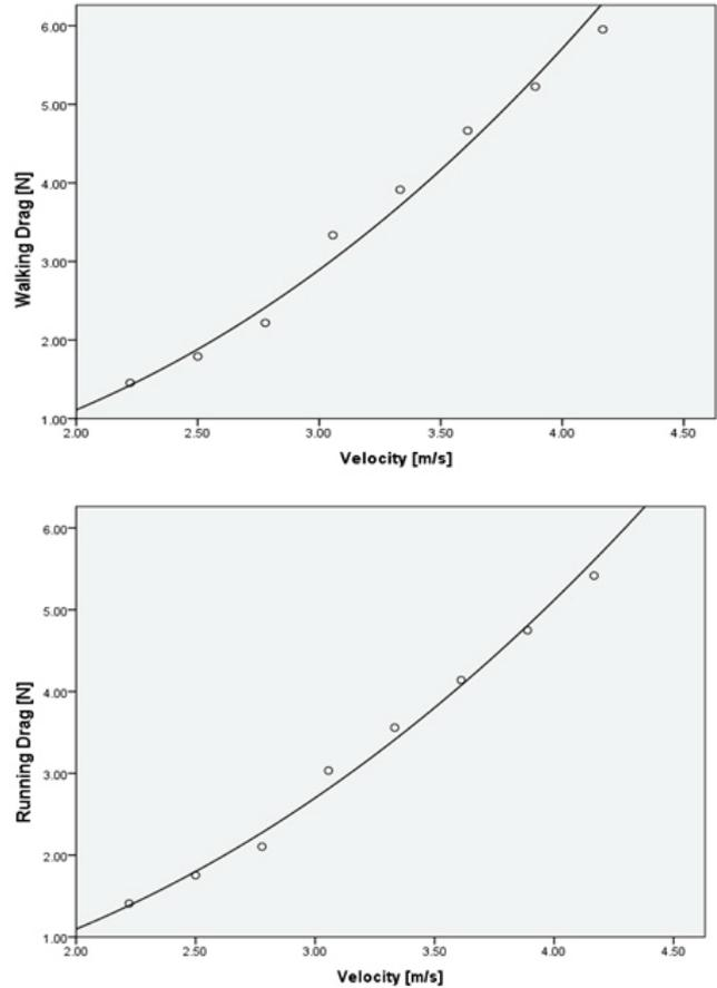
Fig. 8. Trend lines (solid line) for drag variations and with velocity for walking (top panel) and running (bottom panel)
