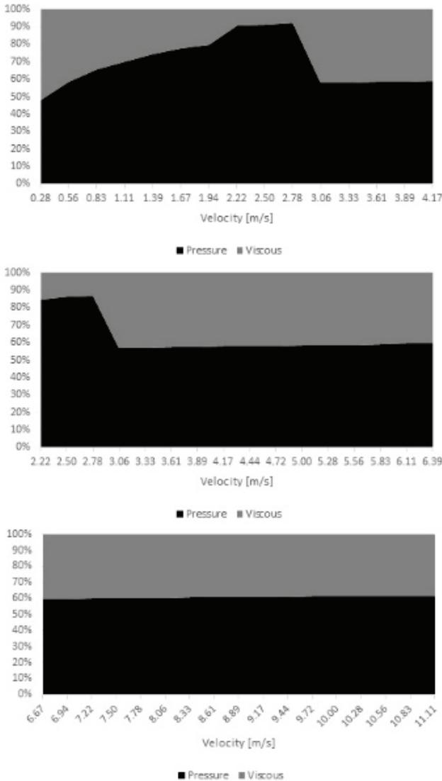
Fig. 7. Contribution of pressure and viscous drag to total drag at the selected velocities for walking (top panel), running (middle panel) and sprinting (bottom panel)
