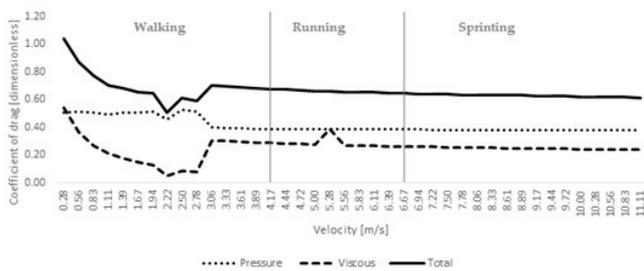
Fig. 4. Pressure, viscous and total drag coefficient from 0.28 m/s to 11.11 m/s for the three locomotion techniques (walking: 0.28–4.17 m/s; running: 4.17–6.39 m/s; sprinting: 6.67–11.11 m/s)
