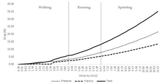
Fig. 5. Pressure, viscous and total drag variations from 0.28 m/s to 11.11 m/s in the three locomotion techniques (walking: 0.28–4.17 m/s; running: 4.17–6.39 m/s; and sprinting: 6.67–11.11 m/s)
