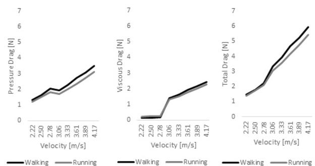
Fig. 6. Pressure (left panel), viscous (middle panel) total drag (right panel) between 2.22 m/s and 4.17 m/s when walking and running
