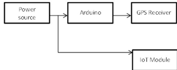
**Fig. 1. Block diagram of GPS based boundary intruding boat monitoring system**
