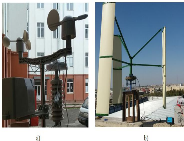
Fig.5. (a) weather station of “MISOL” type, (b)- wind power plant
