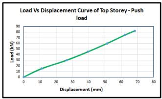
Fig.9Load Vs Displacement curve for RC frame for Top storey – Push type loading
