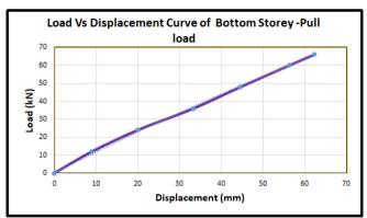
Fig.8Load Vs Displacement curve for RC frame for bottom storey – Pull type loading
