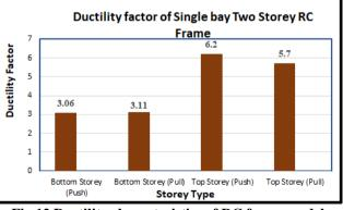
Fig.12 Ductility characteristics of RC frame model
