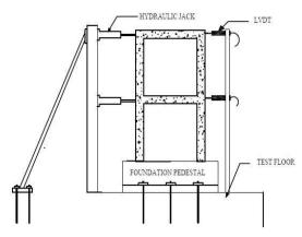
Fig.2 Test Setup of RC Frame Model
