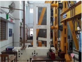
Fig.3Testing of RC Frame Model
