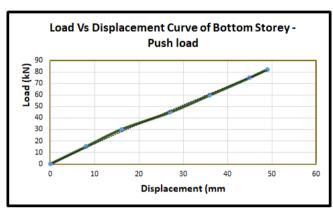
Fig.7Load Vs Displacement curve for RC frame for bottom storey – Push type loading
