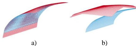
Figure 4. Transverse deflection in the central part of the shell at the beginning of the extension of the double-curvature shell (a) obtained at the first skinning and at the end of the extension by  $12^\circ$  (b)
