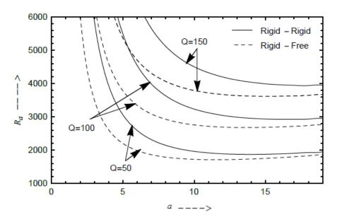
Figure 4. Influence of magnetic field on  $R_a(stat)$  for Q=50,100 and 150 for two different boundaries
