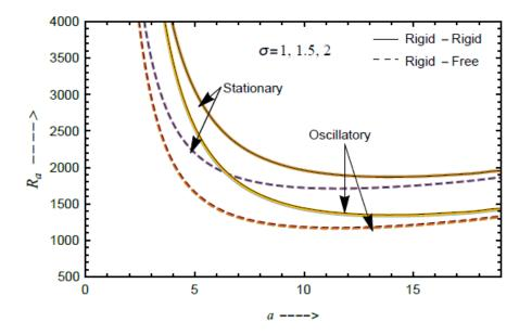
Figure 11. Influence of heat capacity ratio on  $R_a(stat)$  and  $R_a(osc)$  for  $\sigma=1,1.5$  and 2 for three different boundaries
