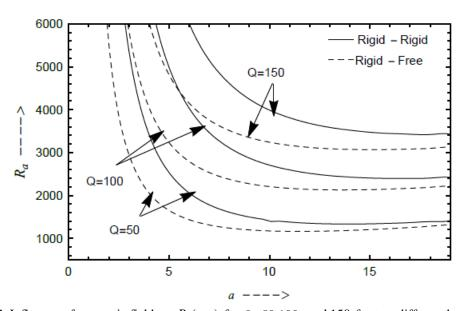
Figure 5. Influence of magnetic field on  $R_a$  (osc) for Q=50,100 and 150 for two different boundaries.
