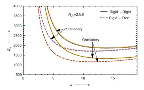
Figure 10. Influence of modified diffusivity ratio on  $R_a(stat)$  and  $R_a(osc)$  for  $N_A=2,5$  and 9 for three different boundaries
