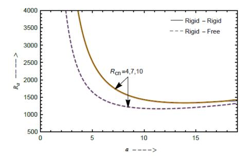
Figure 3. Influence of concentration Rayleigh number on  $R_a(osc)$  for  $R_{cn}=4,7$  and 10 for two different boundaries
