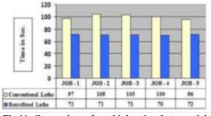
Fig.11: Comparison of machining time between job manufactured on proposed & existing lathe.
