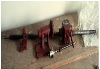
Fig. 3: Lead Screw of X and Z axis
