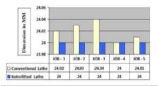
Fig.12: Comparison of job dimension between proposed & existing lathe machine.
