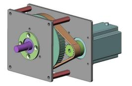
Fig. 6: Assembly of Stepper Motor into Mounting Bracket
