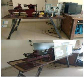
Fig. 10: Developed converted lathe machine
