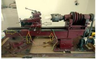
Fig. 8: Limit switches
