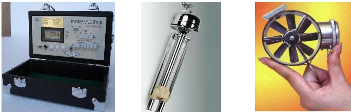
(a) the precision digital barometer      (b) the wet and dry bulb thermometer      (c) the mechanical anemometer
