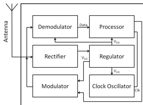
Figure1. Block diagram of passive UHF RFID tag [2]
