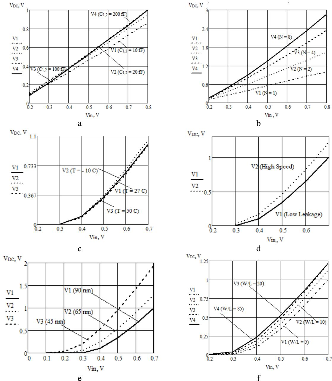
**Figure6.** Simulation results of the voltage rectifier. a – the influence of  $C$  value on the output voltage of 1-stage circuit; b – the output voltage as a function of number of rectifying stages; c – the output voltage as a function of temperature; d – rectified voltage for different types of transistors, e – the output voltage of rectifier under various design rules; f – alteration of ratio  $W/L$  for increasing the output voltage
