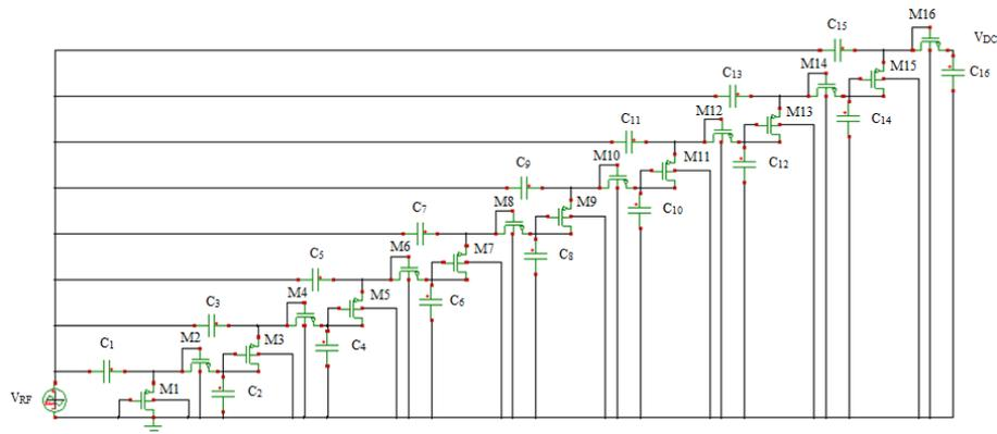
**Figure3.** Schematic circuit of proposed voltage rectifier
