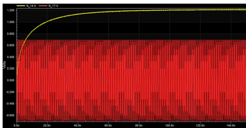
**Figure7.** The transient analysis results of the designed 8-stage rectifier with voltage multiplying at input signal amplitude 0.7 V and frequency 2.45 GHz
