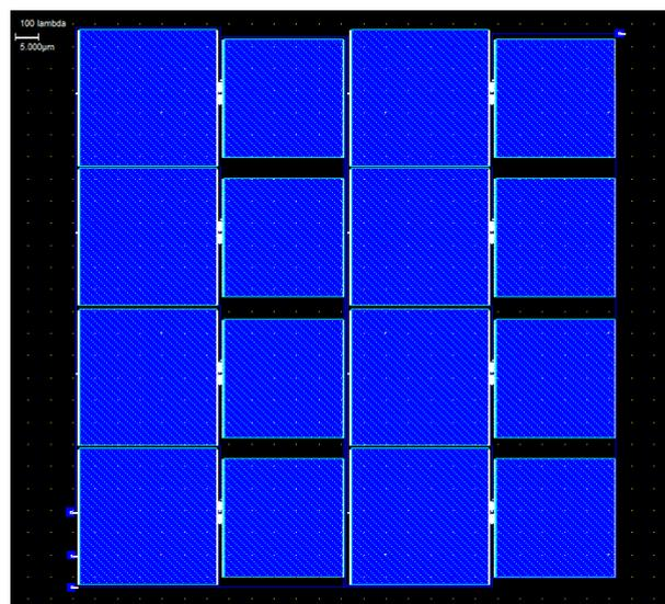
**Figure4.** The layout of rectifier with capacitors performed in 4 metal layers
