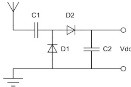
Figure2. Voltage doubler circuit [8]
