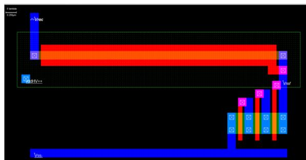
**Figure5.** The layout of reference-voltage source
