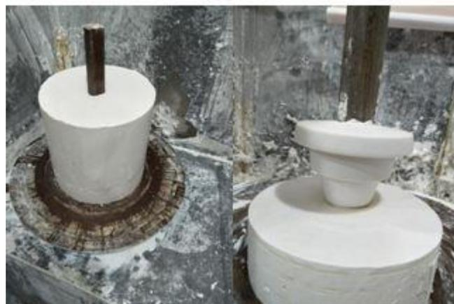
**Fig4.** Jiggering plaster models
