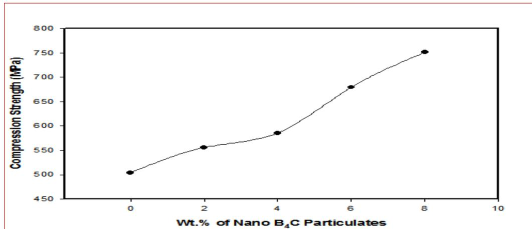
Figure 5 Shows the variation in compression strength of Al2219 alloy and nano composites
