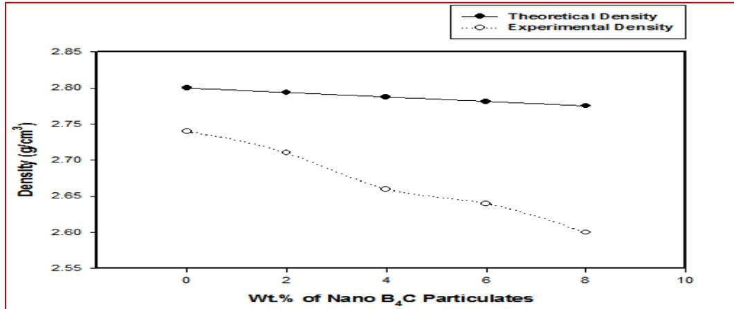
Figure 4 Shows the variation in density of Al2219 alloy and nano composites
