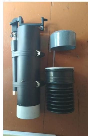
**Fig. 4** PVC pipe covered with insulation tape
