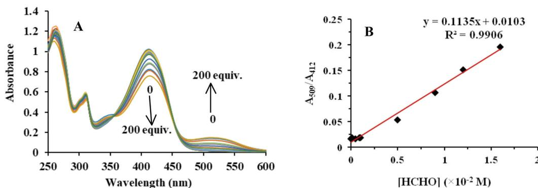
FIGURE 6. The UV-Vis spectra of CHA ( $2.5 \times 10^{-5}$  M) in ethanol with increasing the concentration of formaldehyde (0-200 equiv.) (A). Plot of  $A_{509}/A_{412}$  against concentrations of HCHO (B)
