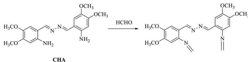
FIGURE 3. Reaction of CHA with formaldehyde in ethanol
