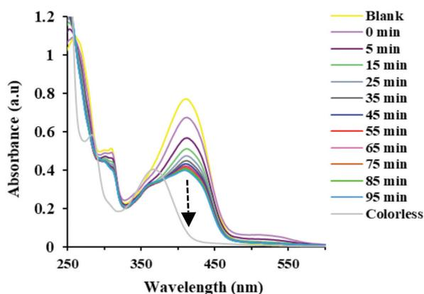
FIGURE 5. Changes in the UV-Vis spectra of CHA ( $2.5 \times 10^{-5}$  M) in ethanol as a time course after addition of formaldehyde solution (200 equiv.) and colorless for 3 h
