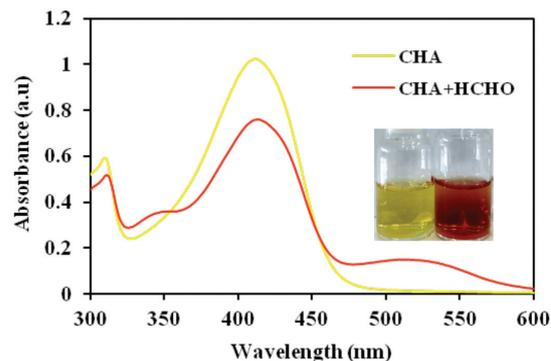
FIGURE 2. The UV-Vis spectra of CHA ( $2.5 \times 10^{-5}$  M in ethanol) before and after addition of formaldehyde (200 equiv.). Inset: Photographs of compound CHA ( $1 \times 10^{-4}$  M in ethanol) before (left) and after addition of formaldehyde (right)
