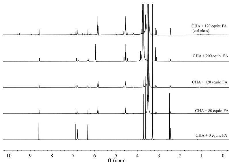
FIGURE 4.  $^1\text{H}$  NMR titration spectra changes of CHA upon addition of formaldehyde in  $\text{DMSO-d}_6$
