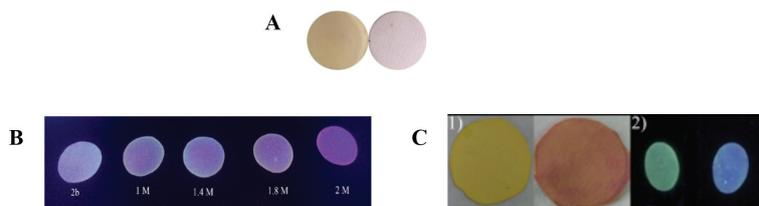
FIGURE 9. Photographs of chemosensor **CHA** ( $1 \times 10^{-3}$  M in ethanol) as paper strip after addition water (left) and formaldehyde (right) in daylight (A), after addition of formaldehyde at various concentrations under 365 nm portable UV lamp (B), and application of meatball test; 1) before and after addition of metball filtrate in colorimetric; 2) before and after addition of metball filtrate in fluorometric (C)
