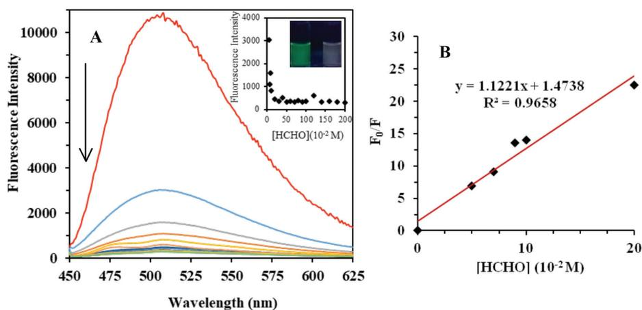
FIGURE 7. Emission spectra of **CHA** ( $2.5 \times 10^{-4}$  M in ethanol) upon addition of formaldehyde in aqueous solution (0-200 equiv.) with excitation at 440 nm. Inset: fluorescence intensity as a function of formaldehyde concentration; photographs of compound **CHA** ( $2.5 \times 10^{-4}$  M in ethanol) before (left) and after (right) addition of formaldehyde under 365 nm portable UV lamp (A). Stern-Volmer plot of **CHA** against concentrations of HCHO (B)
