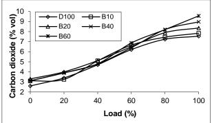
Figure 8 Effect of biodiesel quantity on carbon dioxide emissions Therefore, the  $CO_2$  emissions of the fuels were very close to each other. Higher  $CO_2$  in exhaust emission is an indication of the complete combustion of fuel. This explains the reason for higher exhaust gas temperatures observed (Imdadul, et al., 2016).
