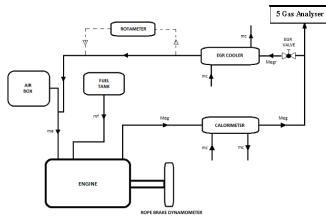
Fig. 3 Line diagram of Engine Experimental setup with Gas Analyzer 2.3 Test Procedure
