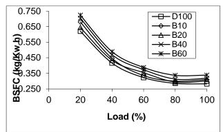
Figure 4 Effect of biodiesel quantity on BSFC
