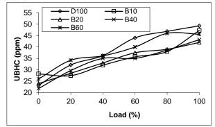
Fig. 10 Effect of biodiesel quantity on emission of UBHC from the engine  $% \left( {{{\rm{D}}{\rm{B}}{\rm{C}}}} \right)$
