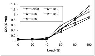
Figure 7 Effect of biodiesel quantity on carbon monoxide emissions
