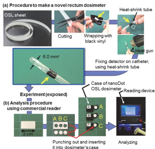
Figure 1. Procedure to make a novel rectum dosimeter and analytical method. (a) Our rectum dosimeter was developed using the OSL sheet, heat-shrink tube, and catheter. (b) The exposed OSL sheet was punched out discs (named A, B and C), and then they were inserted into the dosimeter's case to use a commercial reading device.
