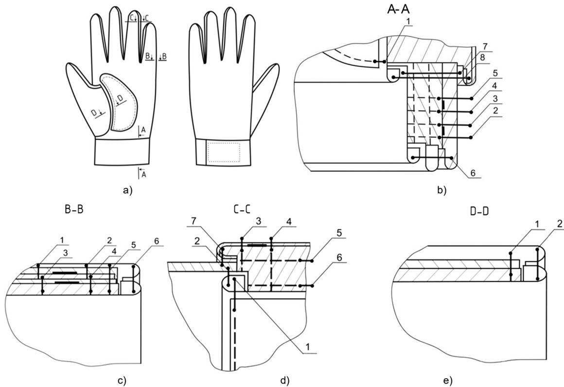
**Figure 7.** The illustrations of methods of technological processing of men's health-saving gloves: (a) location of the cross-sections on the gloves; (b) to cross-section A-A; (c) to cross-section B-B; (d) to cross-section C-C; (e) to cross-section D-D.
