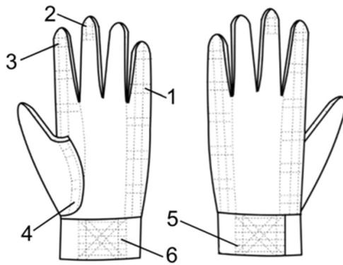
**Figure 6.** The appearance of men's health-saving gloves from the inside out: 1 – the place of the little finger overlay; 2 – the place of the middle finger overlay; 3 – the place of the index finger overlay; 4 – the place of the thumb overlay; 5 – the place of the palmar forearm overlay; 6 – the place of the back forearm overlay.
