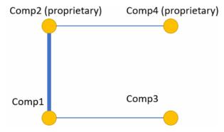
Note: The thick line denotes a proprietary interface; the thin line denotes an open standard.
