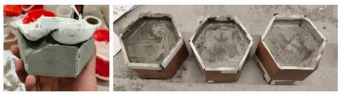
Notes: Illustration of home-produced prototypes using 3D Printed formwork and Concrete. Students develop their designs digitally and use rapid prototyping fabrication services that can deliver materials direct to their home. This material is then used for the manual creation of original works as cast prototypes.
