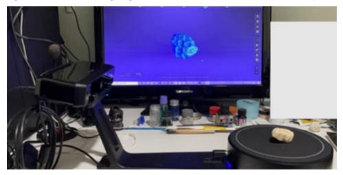
Figure 1 Remote 3D scanning setup from student residence (see online version for colours)
