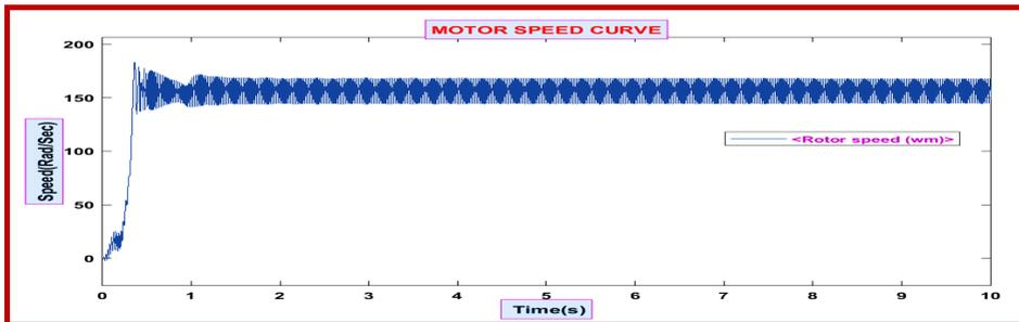
**Figure 6** Speed of inverter-fed asynchronous motor by variation of rotor resistance with PID controller (see online version for colours)
