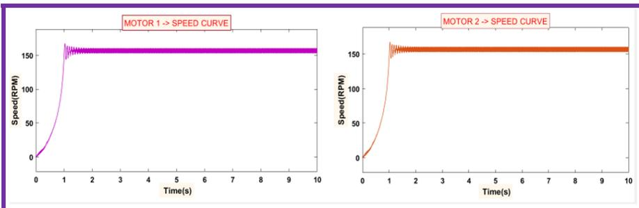
This is the combined speed curve of inverter fed two induction motors connected in parallel using PID controller. This waveform is also analysed by different parameters like settling time, rise time, peak time and delay time. But the speed is same for both the curves is 1475 rpm as given in Figure 11.
