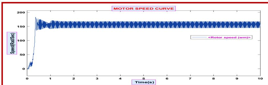
**Figure 7** Speed curve of inverter-fed asynchronous motor by variation of stator resistance with PID controller (see online version for colours)
