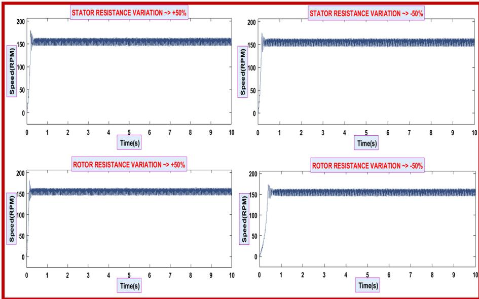
**Figure 18** Speed control of inverter-fed double asynchronous motor with fuzzy controller (see online version for colours)
