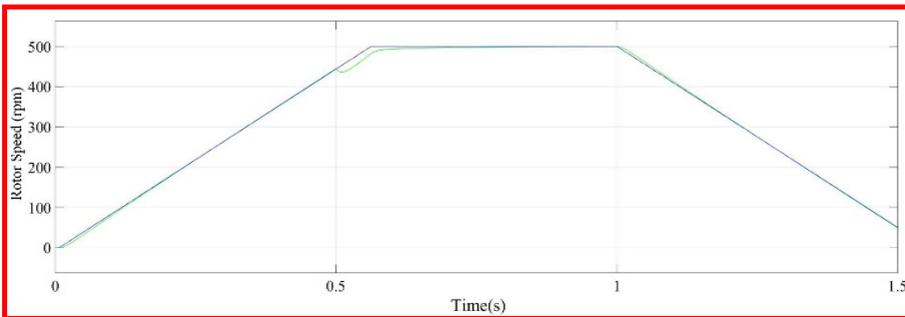
This is the output result of inverter-fed single induction motor using PID controller. The parameters like settling time, rise time, peak time and delayed time are analysed to obtain the output waveform. This result is obtained without variation of parameters as depicted in Table 2.
