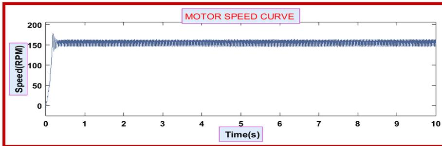
**Figure 16** Speed curve of inverter-fed single induction motor with fuzzy controller by the variation of inertia (see online version for colours)
