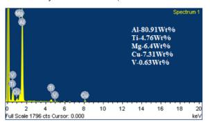
Spectrum analysis indicates that Al content is enhanced to 80.91% whereas Ti content is reduced to 4.76% and results further increase in hardness at 240 mm/min. It is observed that reduction in Ti is not affecting the increasing trend of hardness, as 0.01% Ti is enhanced to 4.76% in Al alloy. This finding is also supported by the higher hardness distribution at fusion zone viewed from the Al side as per Figure 5. Hence, higher welding speed improves the strength of dissimilar weld joints.
