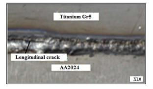
Figure 2 Crack at speed 180 mm/min (see online version for colours)
