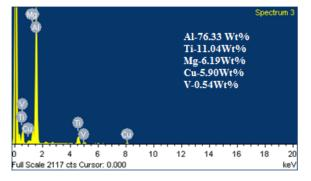
Figure 8 EDS fusion zone analysis at 200 mm/min (see online version for colours)
