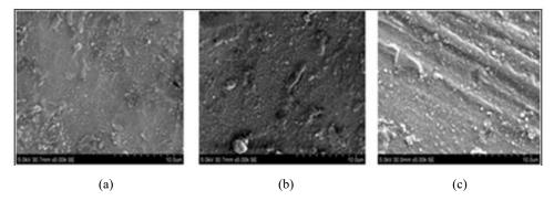
Figure 7(a), Figure 7(b) and Figure 7(c) show fine grain structures at the speed of 240 mm/min. it is noted that grain size decreases with increase in speed. Comparing with weld speed 200 mm/min, at 240 mm/min grain structures are uniformly distributed and are smooth in texture. Thus, higher welding lead to grain refinement both in fusion and HAZs.
