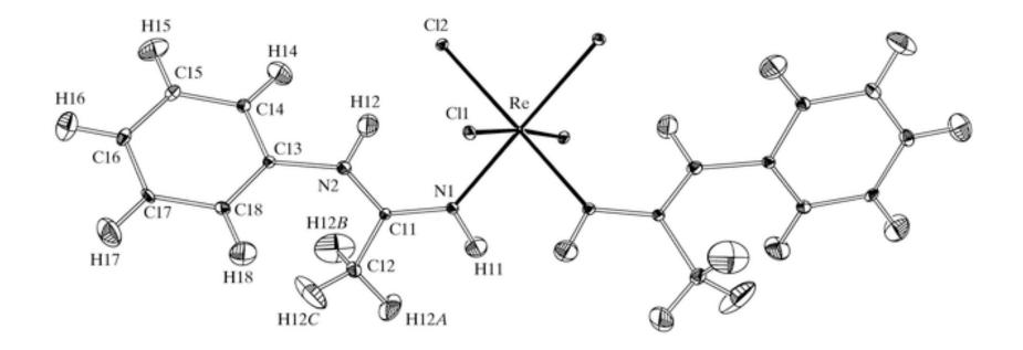
The crystal structure of  $[\text{ReCl}_4(\text{C}_8\text{H}_{10}\text{N}_2)_2]$  at 11 K from X-ray data. Displacement ellipsoids are shown at the 75% probability level. (Figgis et al., *Acta Cryst.* **2001**, *C57*, 1151-1153.)
