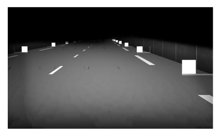
**Figure 4:** Example for a research question considering homogeneity for HD-headlamp systems: defective elements of an image generating device (strongly exaggerated for visualization).
