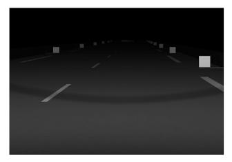
Figure 2: Example for investigated inhomogeneity: annular structure with high negative contrast and small gradient [7].
