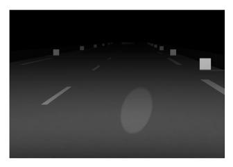
**Figure 1:** Example for investigated inhomogeneity: round structure with high positive contrast and small gradient [7].
