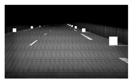
**Figure 3:** Example for a research question considering homogeneity for HD-headlamp systems: projected grid structure of an image-generating device (strongly exaggerated for visualization).
