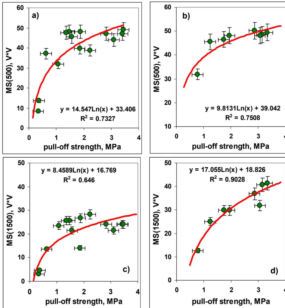
Figure 35. Relationship between mean square value MS and pull-off strength calculated for the VE coating: (a) MS (500  $\mu$ s) and (c) MS (1500  $\mu$ s), and for the PUR coating: (b) MS (500  $\mu$ s) and (d) MS (1500  $\mu$ s).
