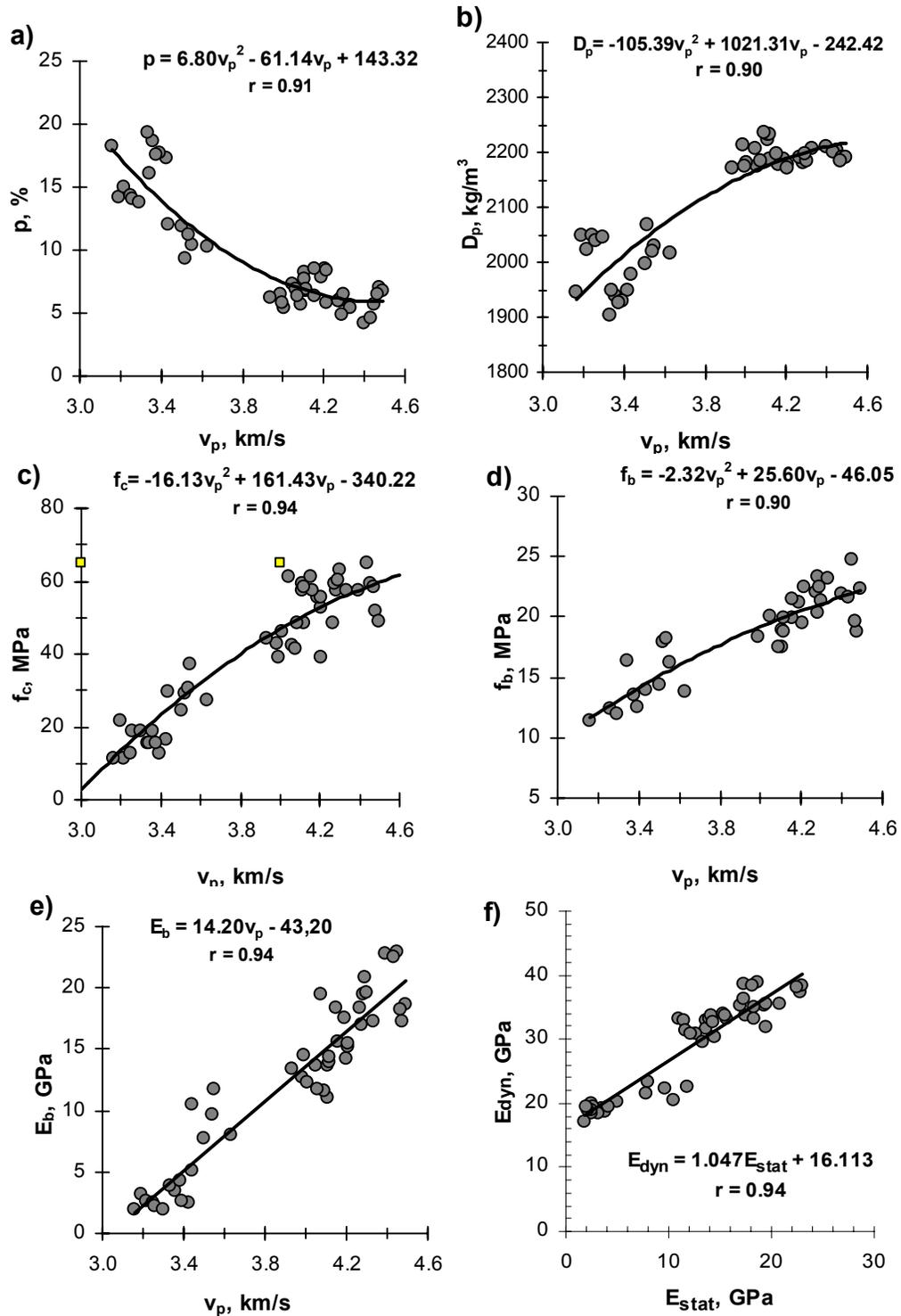
Figure 11. Regression functions describing relationships between the pulse velocity and: (a) porosity,  $p$ , (b) volume density,  $D_v$ , (c) compressive strength,  $f_c$ , d) flexural strength,  $f_b$ , and (e) static elasticity modulus,  $E_b$ , for tested model vinyl ester concretes tested. Graph f) shows the dynamic elasticity modulus,  $E_{dyn}$ , plotted against the static modulus of elasticity,  $E_{stat}$ .
