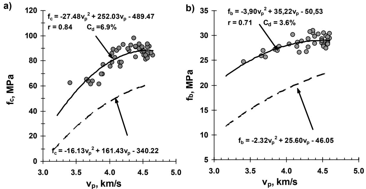
Figure 12. Relationships between pulse velocity,  $v_p$ , and: (a) compressive strength,  $f_c$ , and (b) flexural strength,  $f_b$ , for representative samples of industrial precast elements made from vinyl ester concrete. The dashed line shows the corresponding regression functions for the model vinyl ester concretes, obtained previously (see Table 6).
