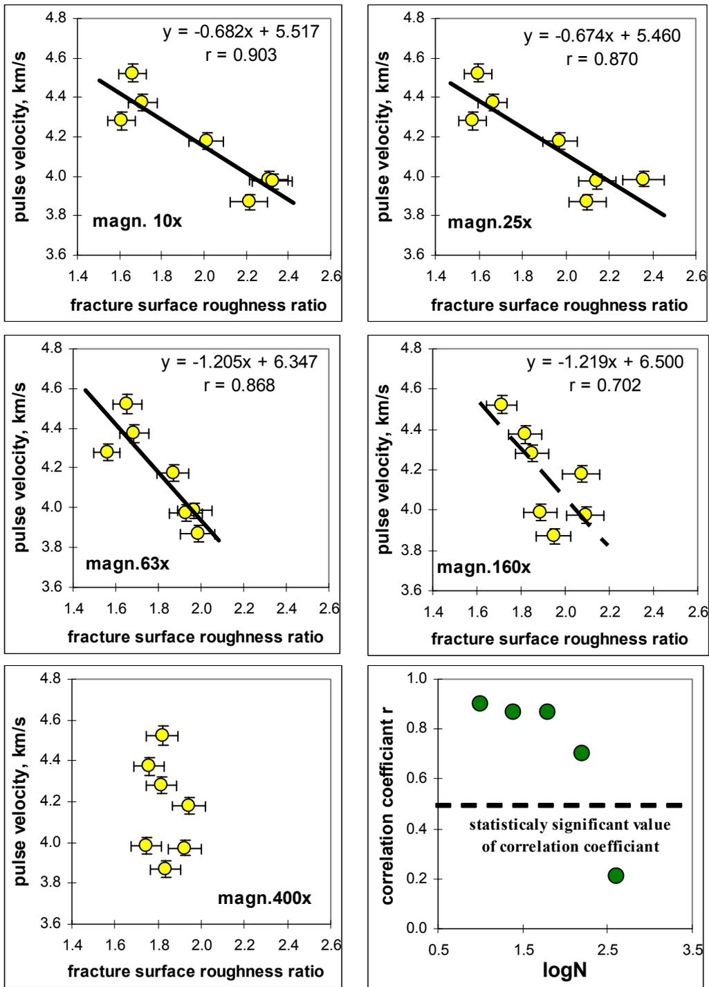
Figure 19. Pulse velocity plotted against surface roughness ratio at different magnifications for epoxy concrete. The correlation coefficient vs. the logarithm base ten of the magnification, N, is also shown.
