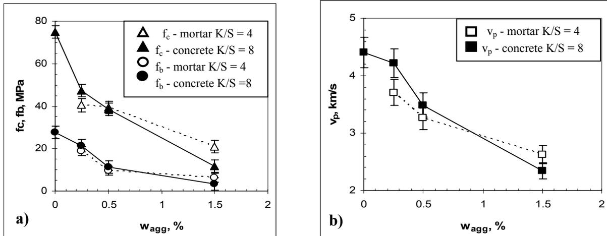
Figure 14. Effect of aggregate moisture content on a) mechanical properties: compressive strength,  $f_c$ , and flexural strength,  $f_b$ , and b) pulse velocity,  $v_p$ , for vinyl-ester mortar and concrete;  $w_{agg}$  – water to aggregate ratio by mass. Error bars represent variation over several nominally identical samples.
