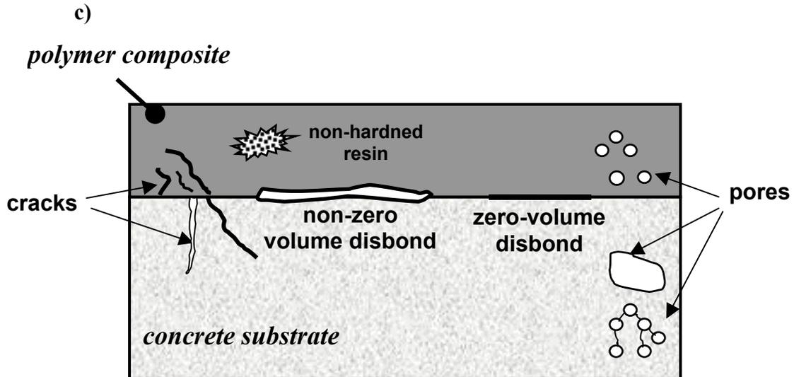
Figure 7. (a) Scheme of determination of reflection coefficient R; (b) R value for common "building interfaces";  $Z_1$ ,  $Z_2$  - acoustic impedance (computed from data in Table 3); (c) sketch of defects in PC-CC system
