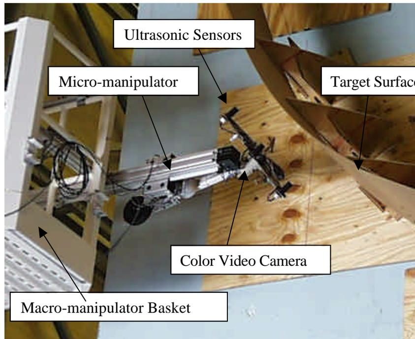
The micro-manipulator carries a small color video camera that provides position feedback to the operator during the experiment. A paper target with regularly spaced sets of colored lines cover the target surface. The position of those lines on the video screen comprises the position feedback. A Macintosh 7600/120 computer running Avid VideoShop records the video images for subsequent evaluation.
