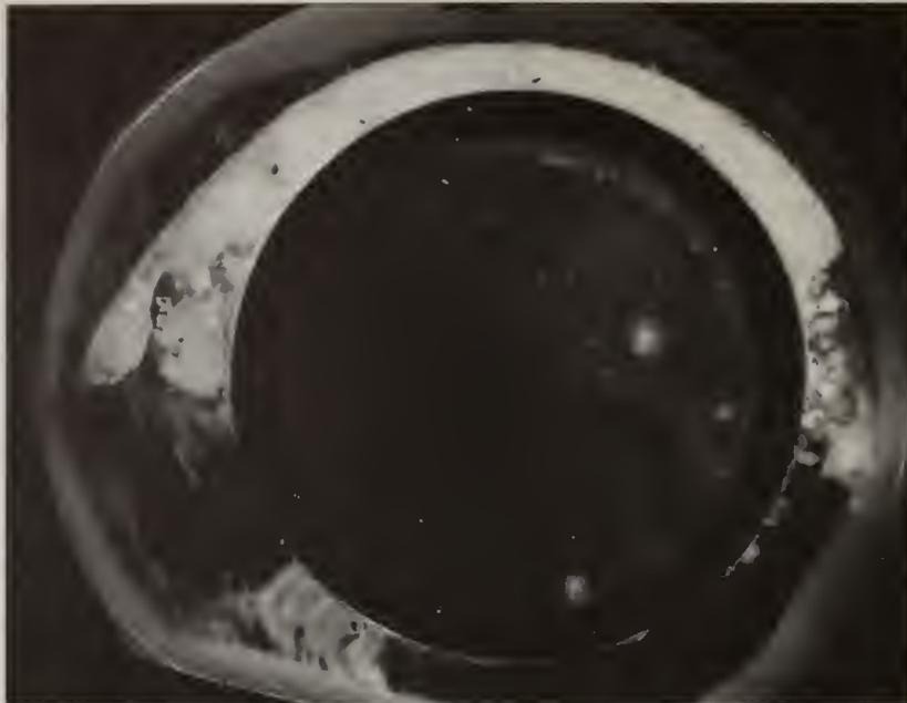
Fig. 3. Section of Type 316 stainless steel tubing after exposure to  $K_2SO_4 + K_2CO_3$  seeded  $O_2$  rich hot gas stream. Note thick deposit on upper surface. Tube temperature  $500\text{ }^\circ\text{C}$ . 6 X.
