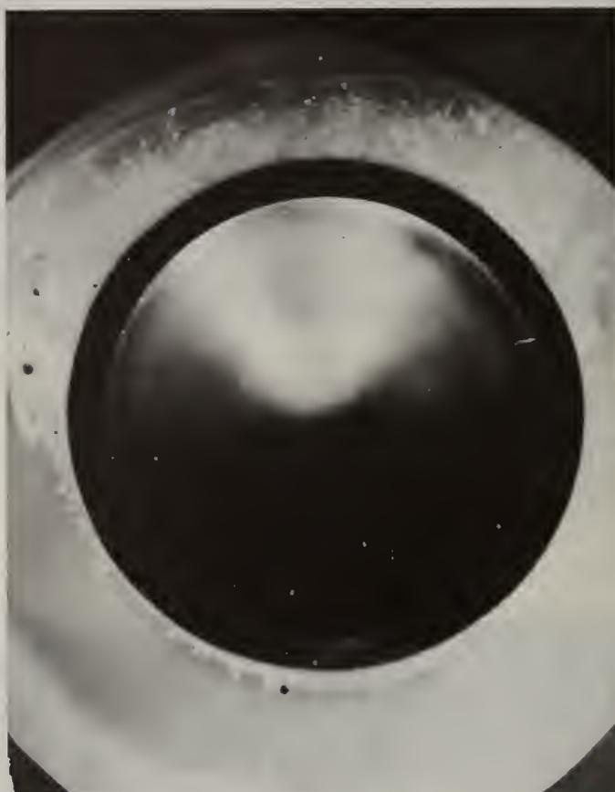
Fig. 7. Section of Type 304 stainless steel tubing after exposure to  $K_2SO_4$  seeded oxygen rich hot gas stream. Note formation of thick deposit, 2 mm, on upper surface and thin powdery deposit on lower surface. Tube temperature 400 °C. 6 X.
