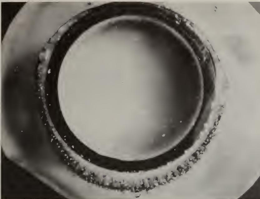
Fig. 12. Section of Type 304 stainless steel tubing after exposure to  $K_2SO_4$  seeded fuel rich hot gas stream. Tube temperature  $590^\circ C$ . 6 X.
