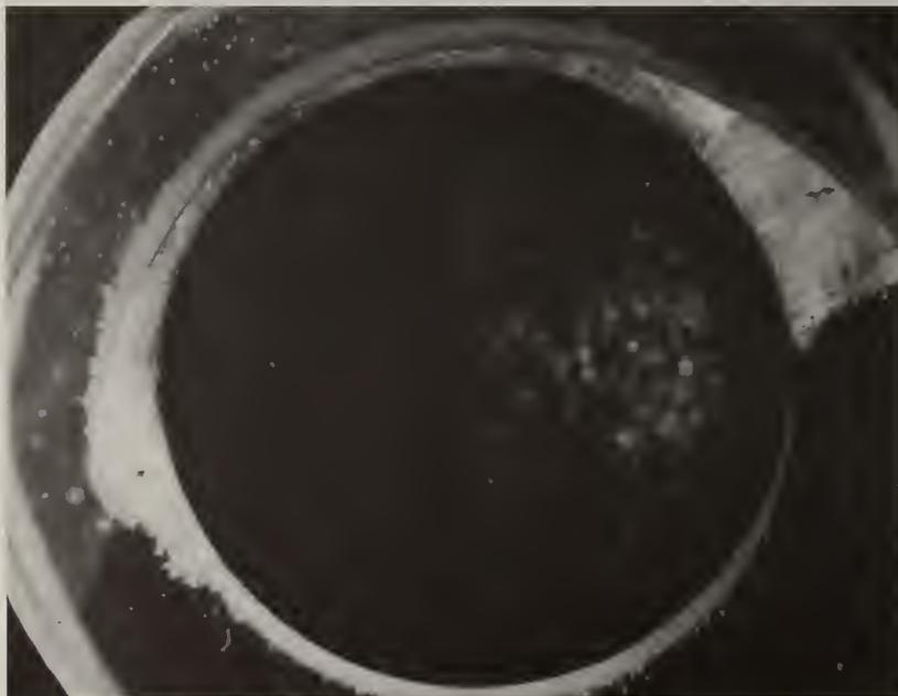
Fig. 15. Section of Type 304 stainless steel tubing after exposure to  $K_2SO_4 + K_2CO_3$  seeded oxygen rich hot gas stream. Note formation of thinner deposit on upper surface. Tube temperature 590 °C. 6 X.
