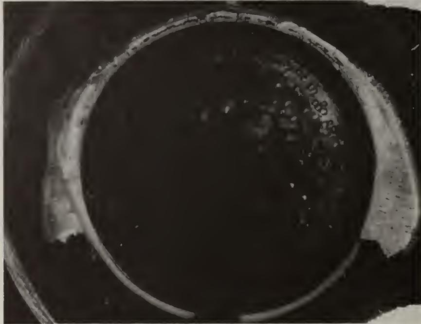
Fig. 18. Section of Type 304 stainless steel tubing after exposure to  $K_2SO_4 + K_2CO_3$  seeded fuel rich hot gas stream. Note deposit on lower surface. Tube temperature 590 °C. 6 X.
