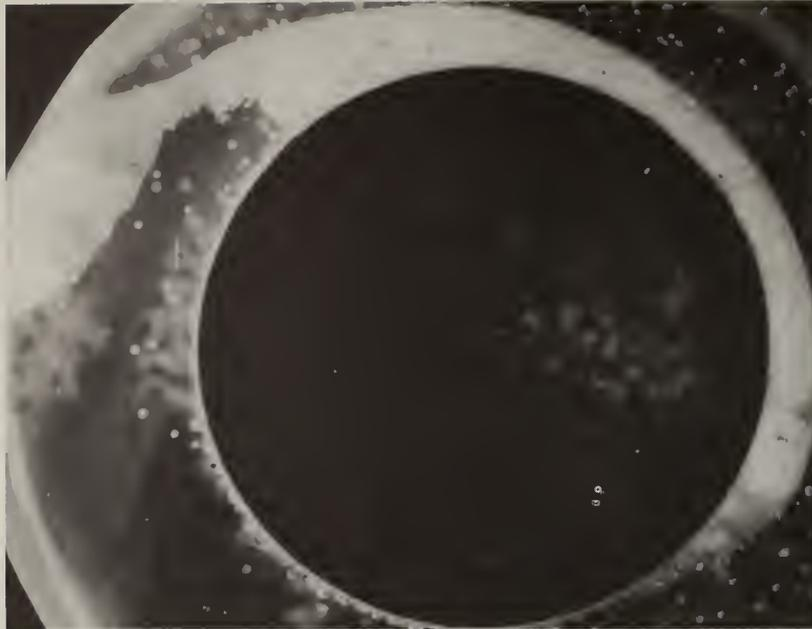
Fig. 14. Section of Type 304 stainless steel tubing after exposure to  $K_2SO_4 + K_2CO_3$  seeded oxygen rich hot gas stream. Note formation of thick, 1 mm, deposit on upper surface. Tube temperature 500 °C. 6 X.
