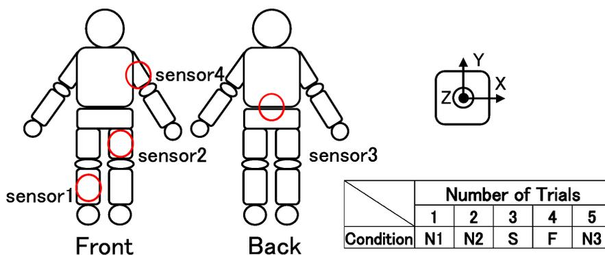
FIGURE 1. The sensor setting: a subject's body, three-axis of local coordinate on accelerometer module and walking condition
