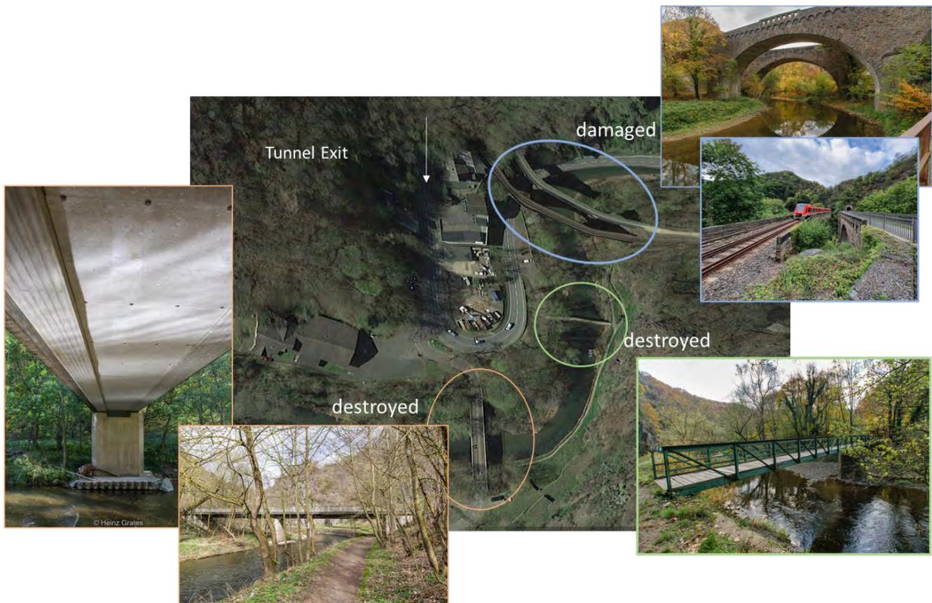
Figure 3.163. google maps excerpt of tunnel exit and surrounding bridges, two of which were washed away. Before flood photos: Heinz Grates, Source: [https://www.aw-wiki.de/index.php/Ahrbr%C3%BCcken\\_im\\_Kreis\\_Ahrweiler](https://www.aw-wiki.de/index.php/Ahrbr%C3%BCcken_im_Kreis_Ahrweiler)
