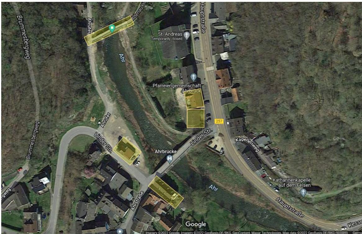
Figure 3.101. Location of Brück and highlighted structures along and across the Ahr which were completely missing (washed away)
