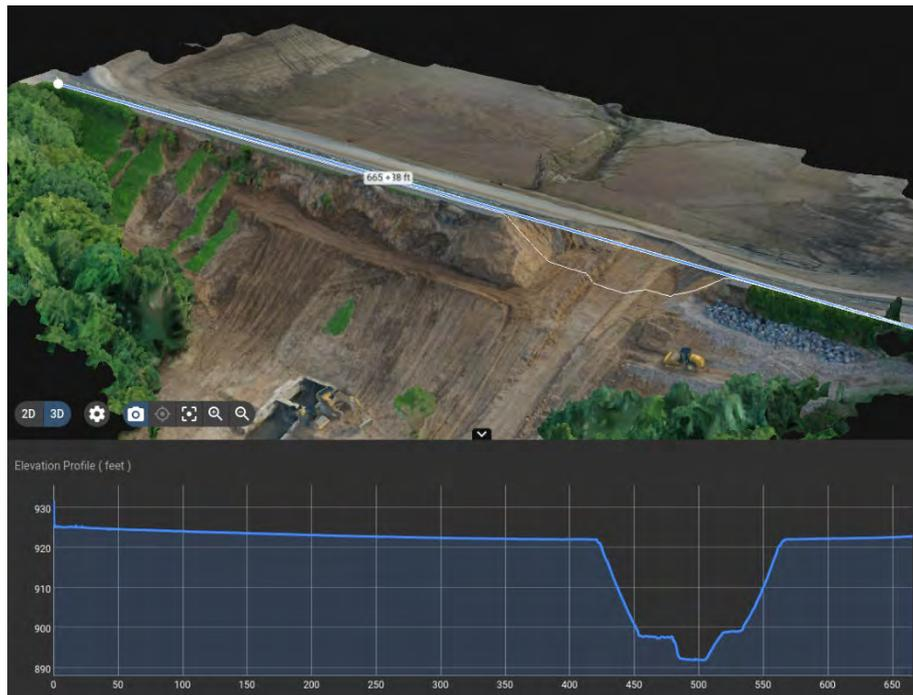
Figure 2.4. Structure for Motion model of Steinbachtalsperre
