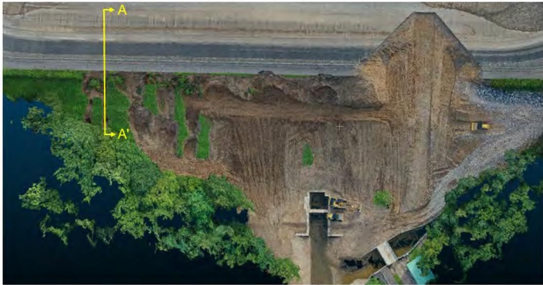
Figure 3.52. Cross-section of scoured gully on the downstream face of the Steinbachtalsperre showing step-pool geometry. Cross-section developed from the SfM model.
