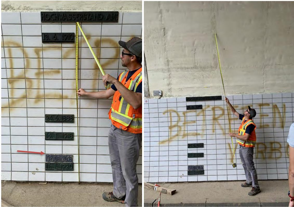
Figure 3.157. Water elevation markers inside the Altenahr tunnel (left) and estimated water level during the 2021 flood event (right); (50.51631664, 6.9968335).
