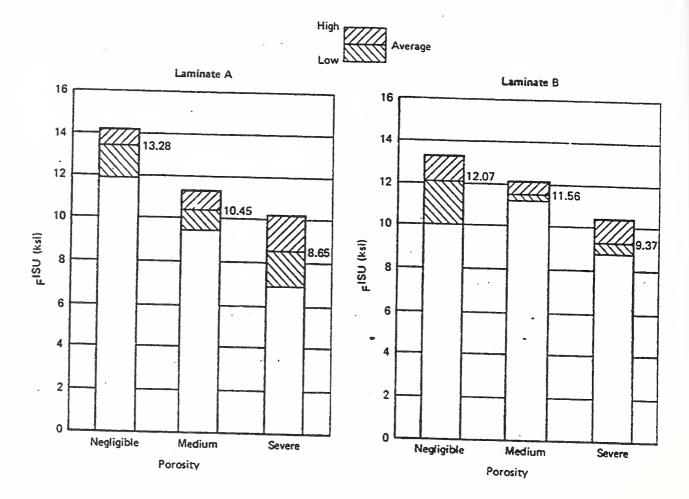
FIGURE 5-20 EFFECTIVE OF POROSITY ON LAMINATE A AND B STATIC INTERLAMINAR SHEAR STRENGTH R.T./Dry
