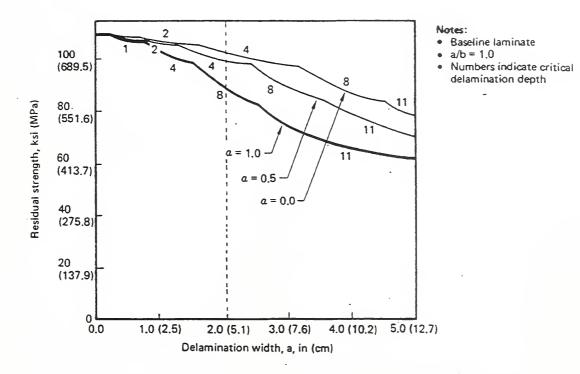
Figure 3-24. Influence of Boundary Fixity on Laminate Static Strength
