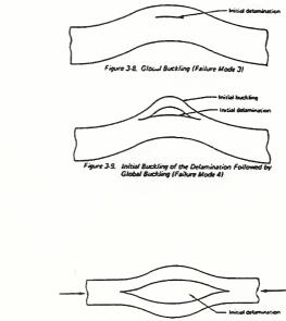
Figure 3-10. Local Buckling (Failure Mode 5)
