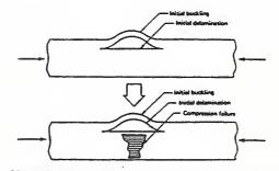
Figure 3-7. Initial Buckling of the Delamination Followed by Compression Failure (Failure Mode 2)
