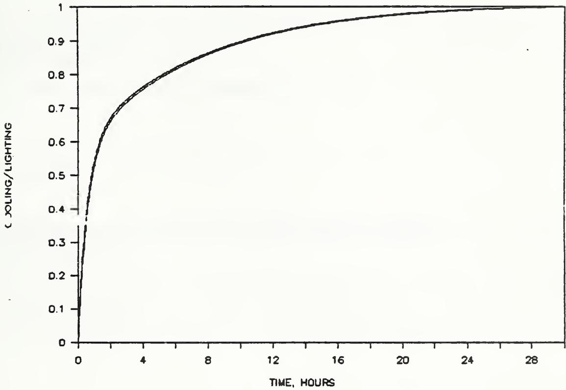
Figure 25. Normalized cooling load profile with 3 percent offset
