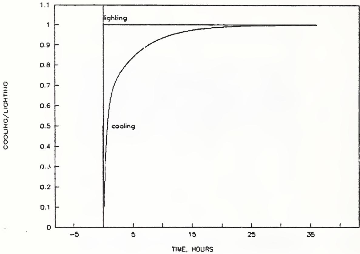
Figure 14. Cooling load profile with no excess heat gains or heat sources
