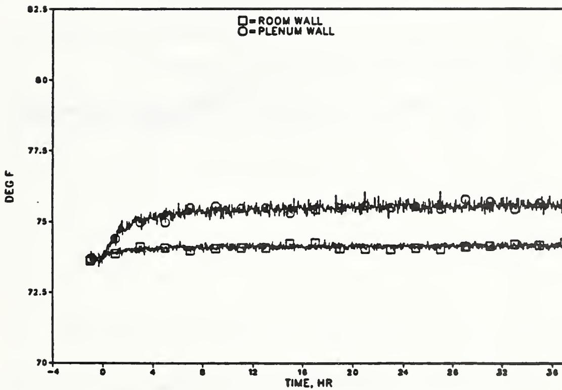
Figure 9. Measured room and plenum wall temperatures for a transient lights-on test
