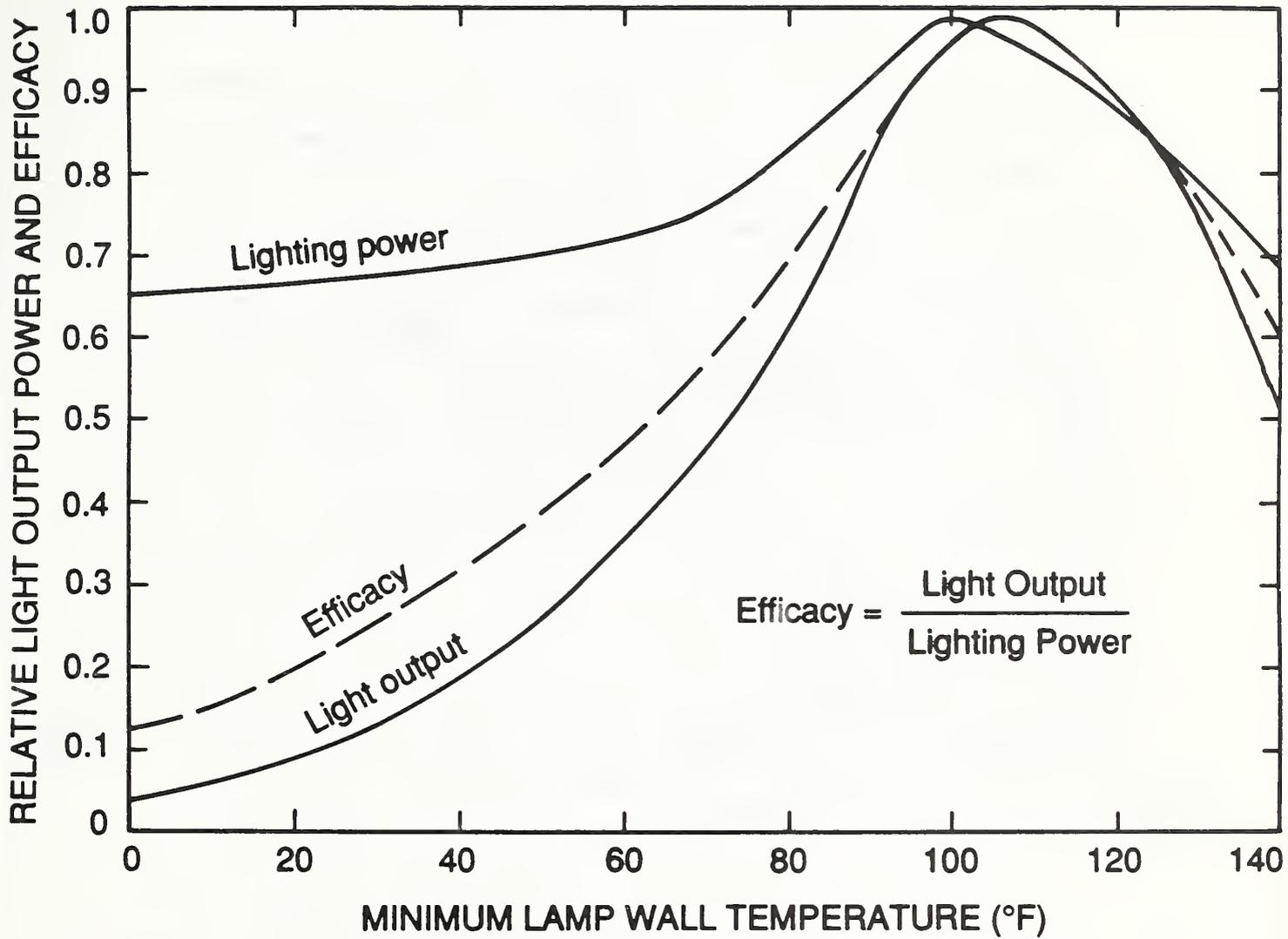
Figure 3. Temperature dependence of a typical fluorescent lamp
