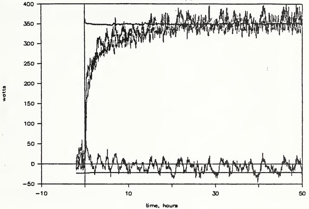
Figure 23. Measured cooling load adjusted using heat flow sensors vs. equilibrium calibration
