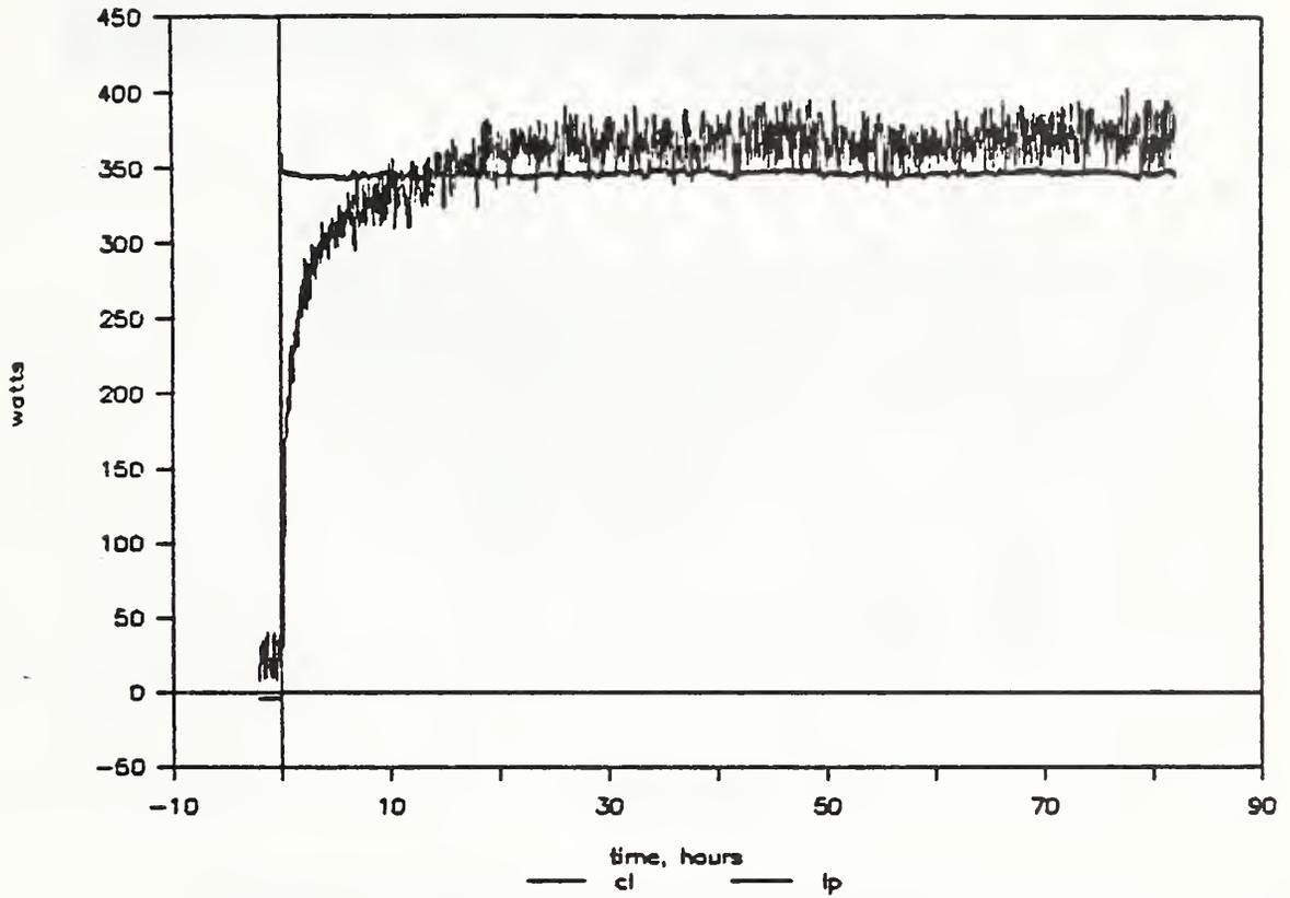
Figure 17. Measured lighting power and cooling load for transient test showing zero and full scale offsets
