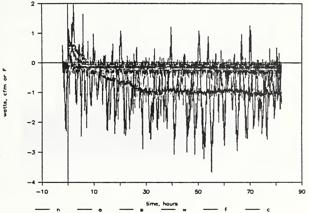
Figure 19. Wall and slab heat flow sensor readings
