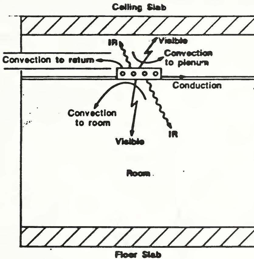
Figure 1. Energy distribution fractions from lighting systems
