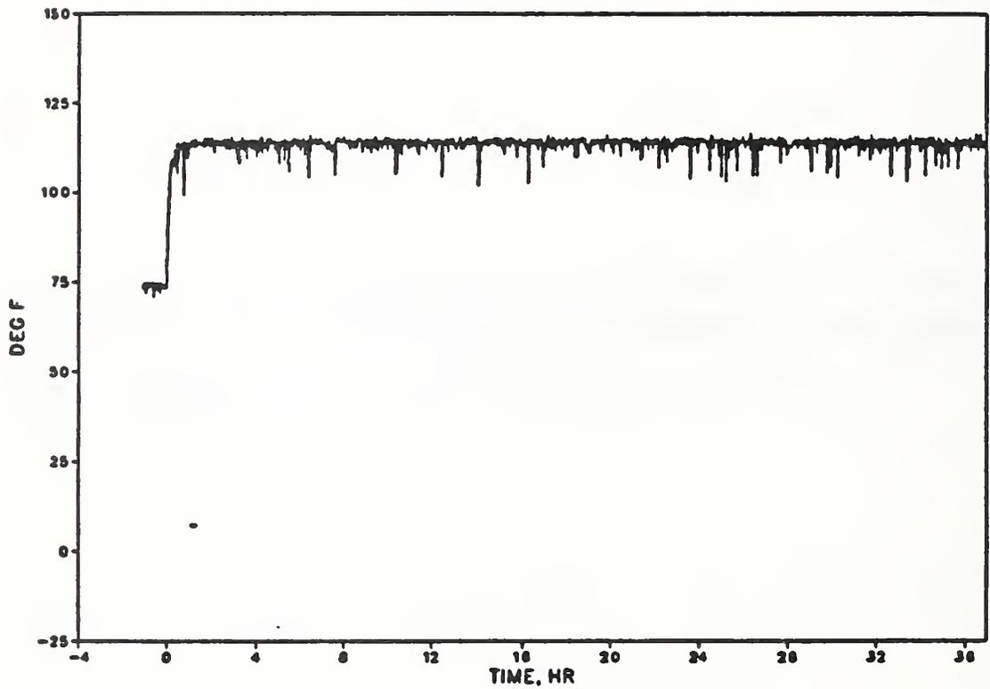
Figure 10. Measured minimum lamp wall temperature for a transient lights-on test
