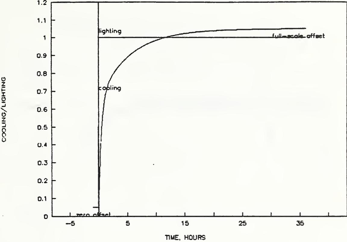
Figure 15. Cooling load profile with constant auxiliary heat source
