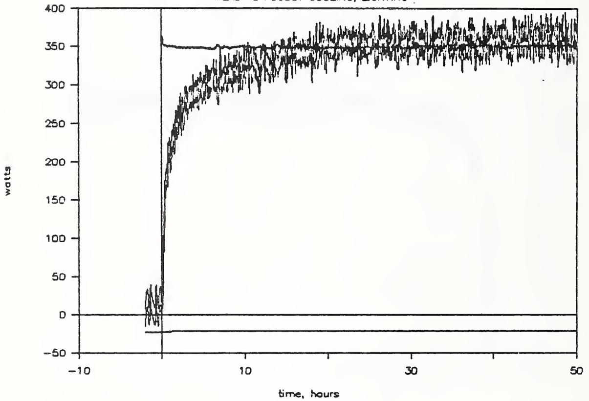
Figure 18. Measured cooling load adjusted for excess heat gains
