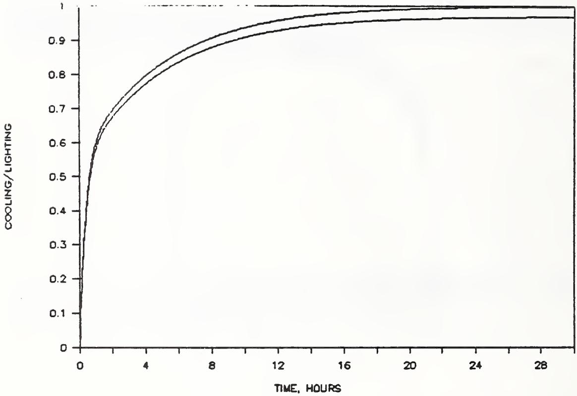
Figure 24. Cooling load profile with 3 percent offset
