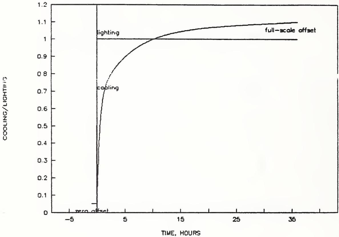
Figure 16. Cooling load profile with variable auxiliary heat source
