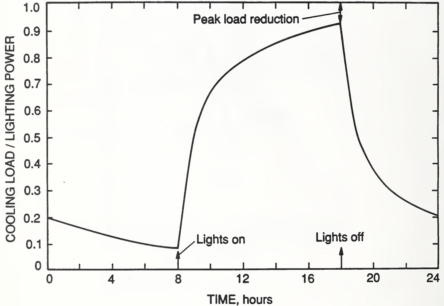
Figure 2. Typical profile of cooling load due to lighting for cyclic daily operation of the lights
