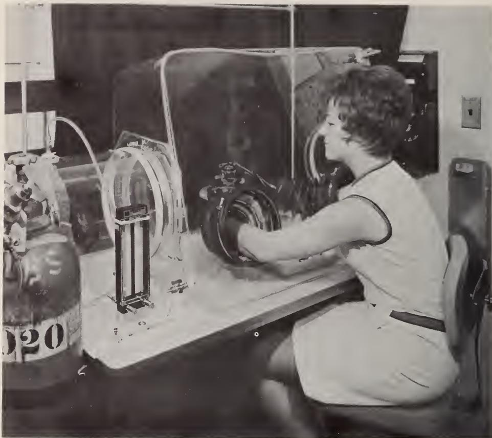
Figure 42. Glove box setup for lithium sample preparation.
