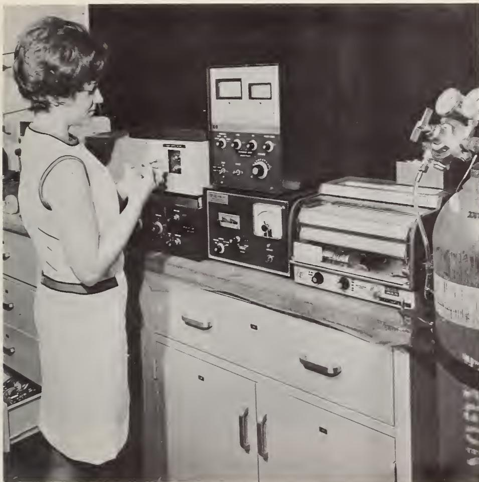
Figure 41. Gas chromatograph with thermal conductivity detector.
