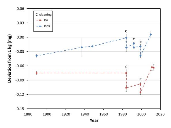
**Fig. 1.** History of the calibration of the U.S. National Prototype K20 and check standard K4 at the BIPM. The uncertainty bars (k=1) for each number are the uncertainties reported by the BIPM on the calibration certificates. No uncertainty was reported on the 1948 calibration of K20.
