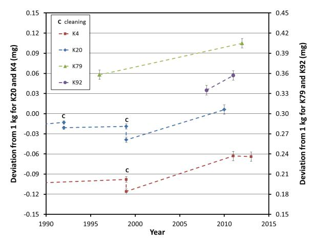
Fig. 2. History of the calibration of all four Pt-Ir prototypes at the BIPM since 1990. The K4 and K20 data is identical to the last three calibrations shown in Fig. 1. The uncertainty bars (k=1) for each number are the uncertainties reported by the BIPM on the calibration certificates.
