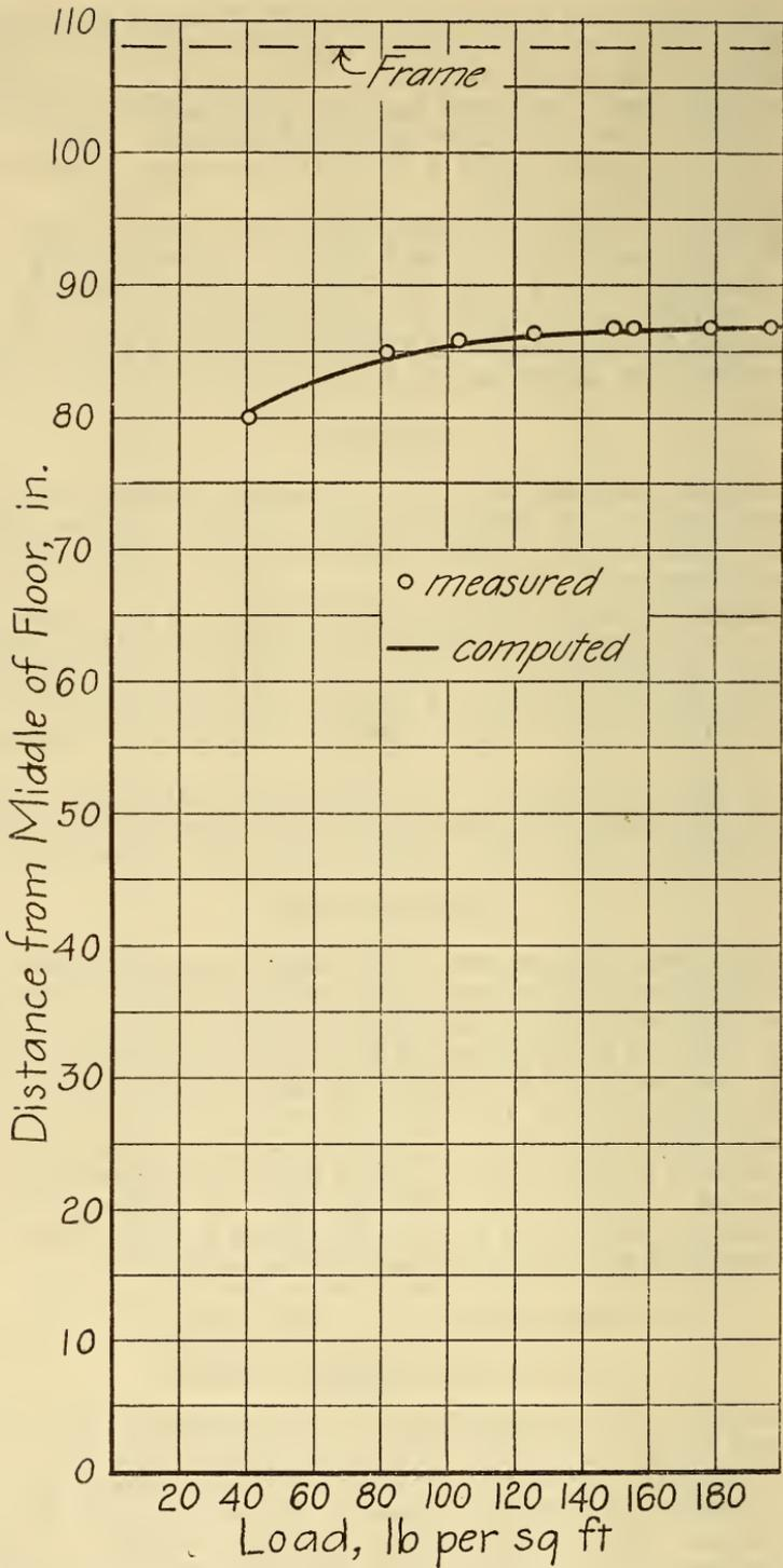
FIGURE 7.—Movement of the point of zero stress along the bottom flange of beam no. 4 as the load increased.
