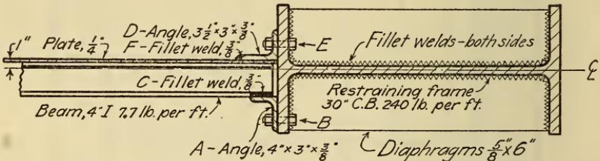
FIGURE 3.—A longitudinal section at the end of the floor.
