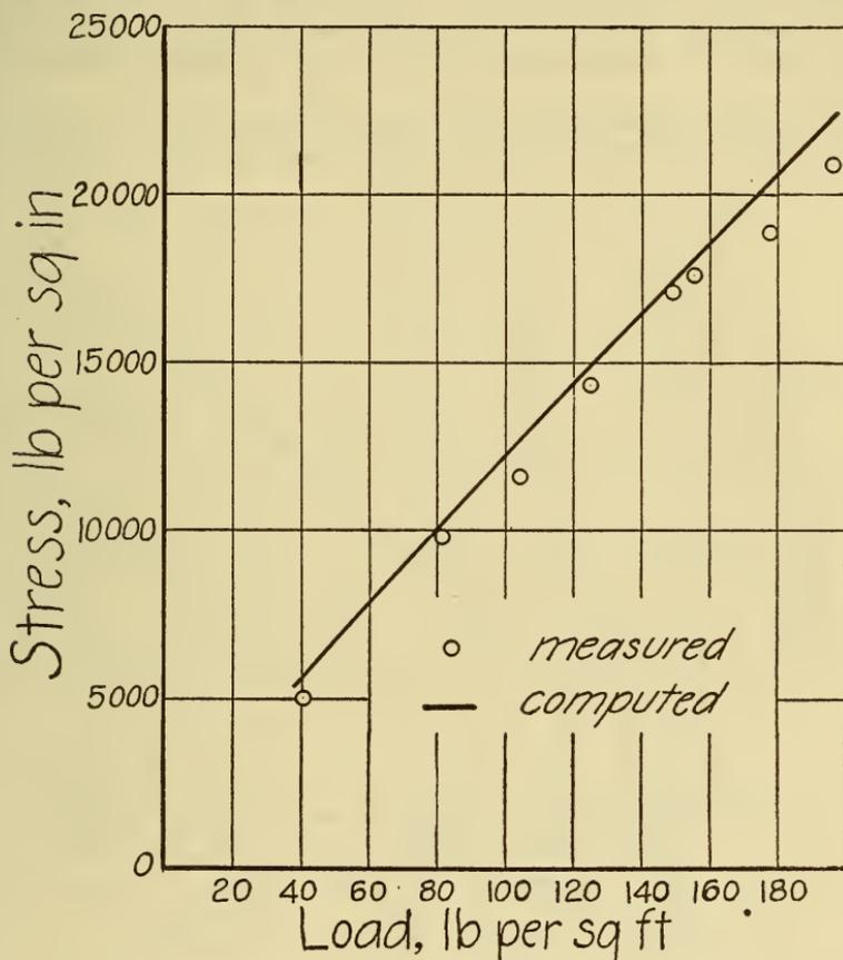
FIGURE 8.—Stresses in the bottom flange of beam no. 4 at midspan.
