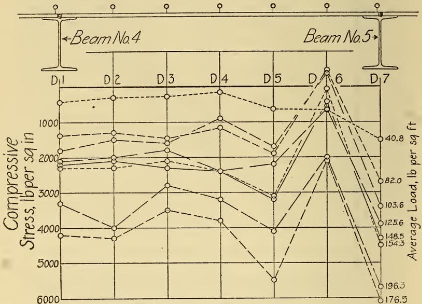
FIGURE 13.—Longitudinal stresses at midspan in the plate between beams nos. 4 and 5.
