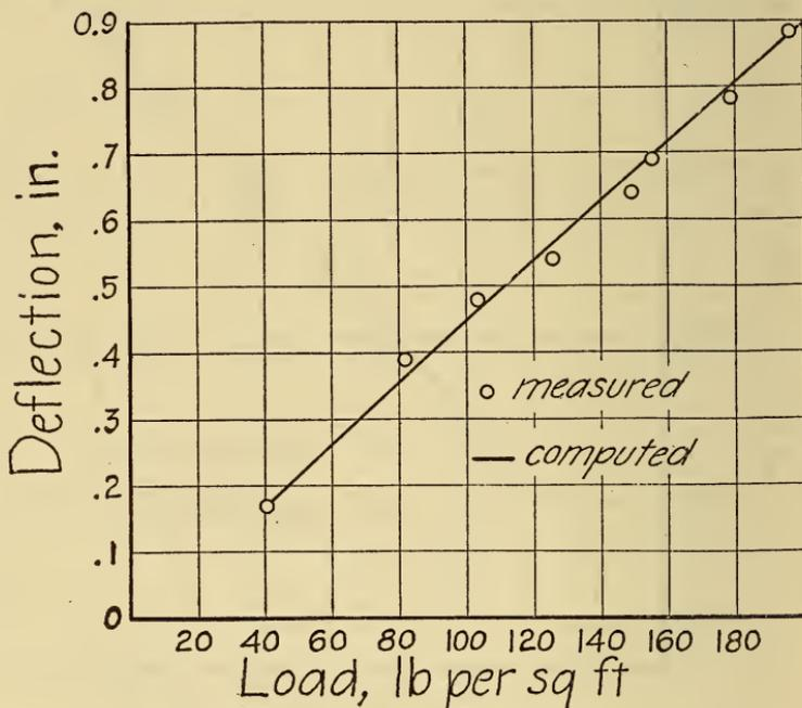
FIGURE 9.—Deflections of beam no. 4 at midspan.
