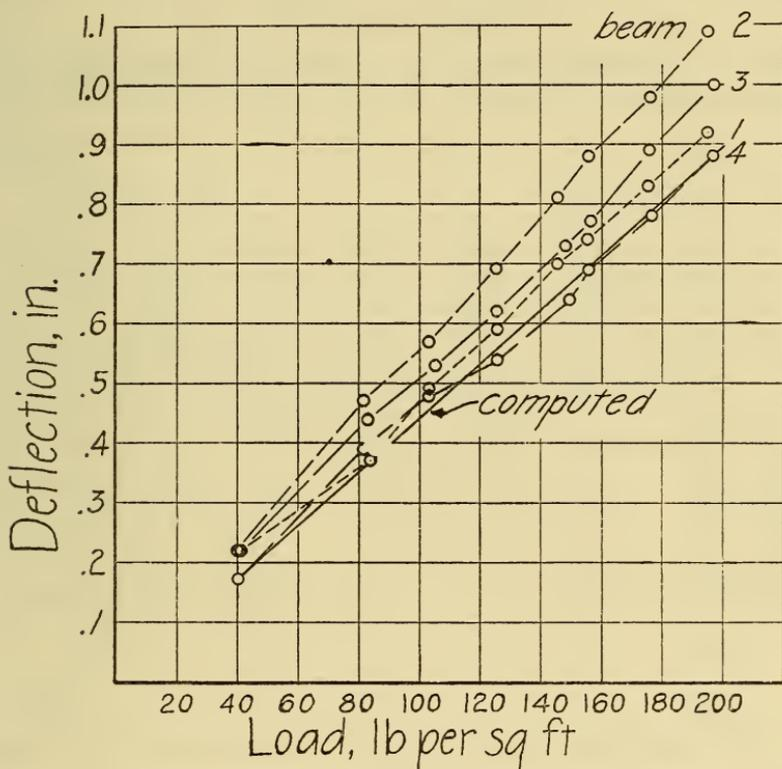
FIGURE 12.—Measured deflections at midspan for beam elements nos. 1, 2, 3, and 4
