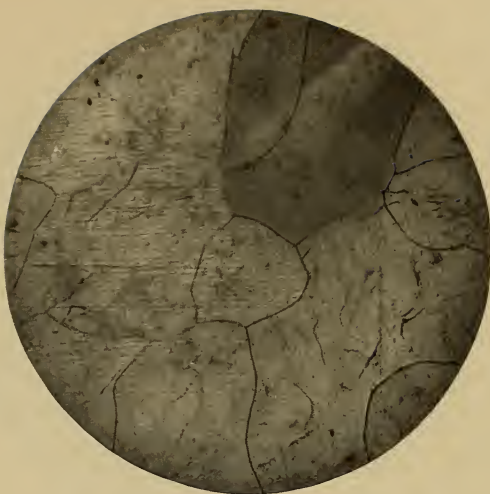
FIG. 2.—C. F. Burgess's electrolytic iron heated to 1050° C several times but not remelted
